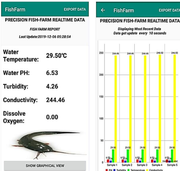
Figure 7. Developed App. Frontend and Graphical View of the Sensed Data
