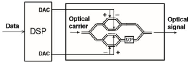
Figure 11. DSP based optical transmitter
