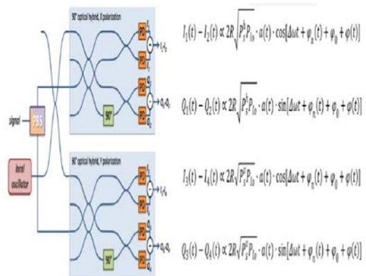
Figure 16. PD coherent receiver
