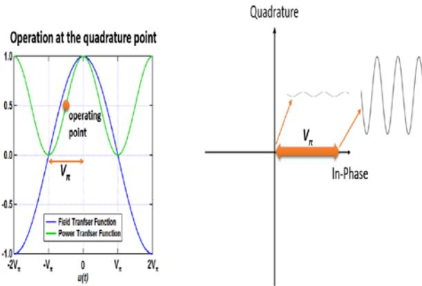
Figure 6. Operation at Quadrature point
