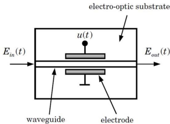
Figure 3. Device structure of phase modulation
