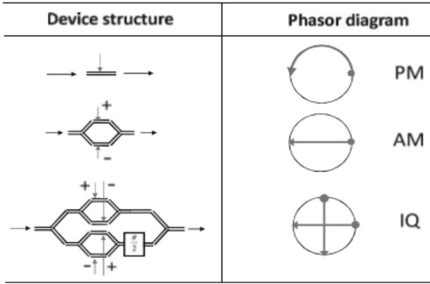
Figure 2. Device structure and the phasor diagram comparison among phase modulation, amplitude modulation, and IQ modulation.
