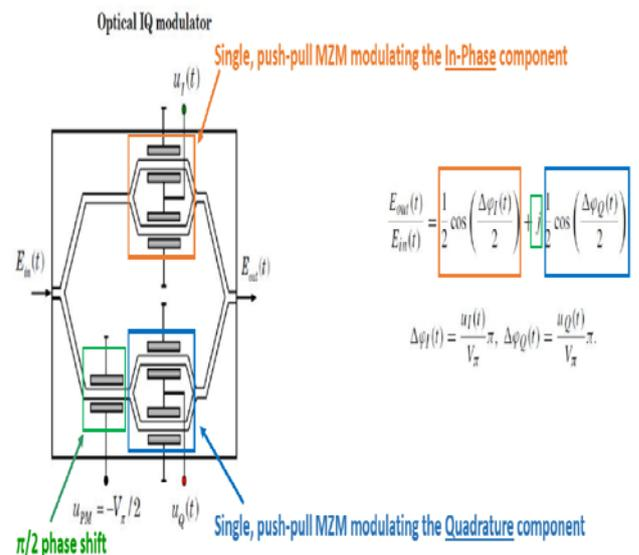
Figure 9. Dual-Nested IQ (In-Phase, Quadrature) Mach-Zehnder Modulator (with each MZM biased at minimum transmission point)
