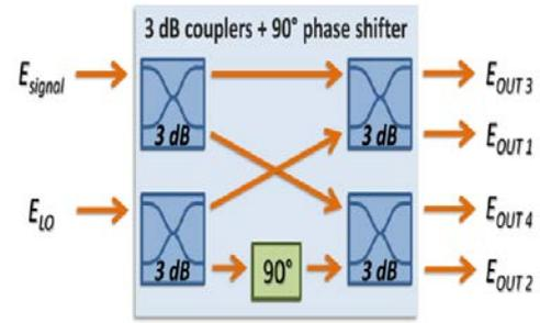
Figure 14. 3dB coupler with 90 degree phase shift
