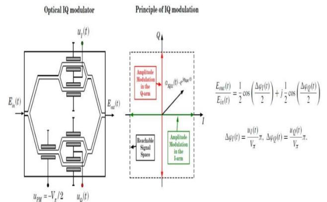
Figure 10. Dual-Nested IQ (In-Phase, Quadrature) MZM (with each MZM biased at minimum transmission point) and principle behind it.
