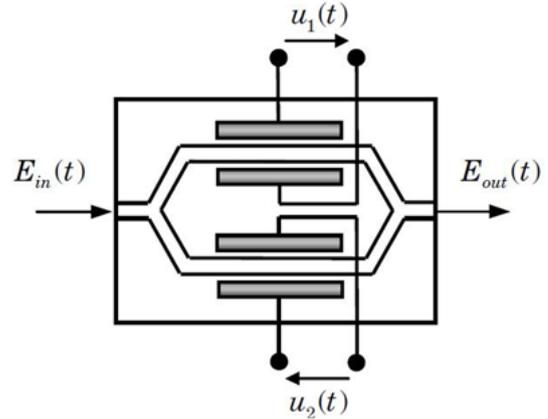
Figure 4. Device structure of MZM
