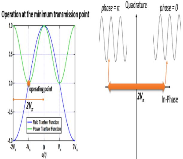
Figure 7. Operation at minimum point
