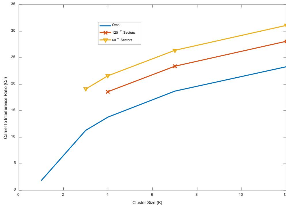
**Figure 5.** Variation of Cluster Size (K) with Carrier to Interference Ratio(C/I) for Omni, 120° Sectors and 60° Sectors
