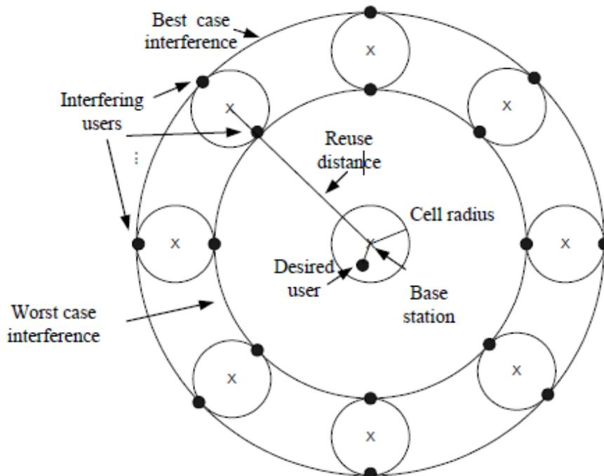
Figure 2. System model for spectral efficiency
