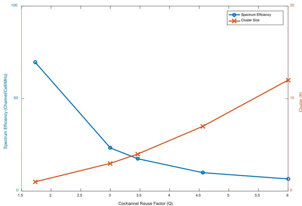
**Figure 4.** Variation of Co-Channel Reuse Factor with Spectrum Efficiency and Cluster Size for Omni and sectors cell
