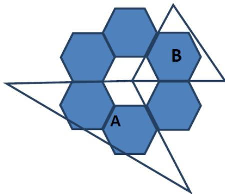
Figure 3. Two Sectors with different Angles, A: $120^\circ$  and B: $60^\circ$  showing the Interferers in each case [12]
