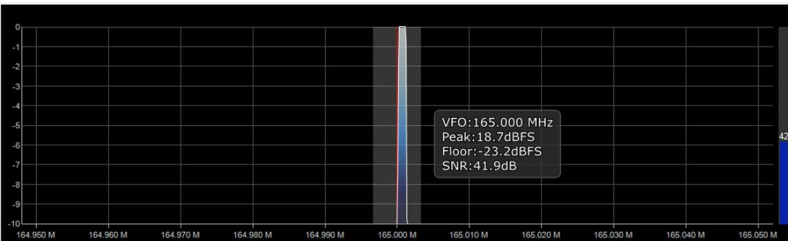
Figure 5. Signal strength when the transmitter facing the right parasitic element shorted by capacitor
