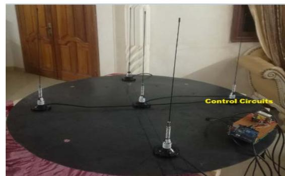
Figure 1. The RDF setup
