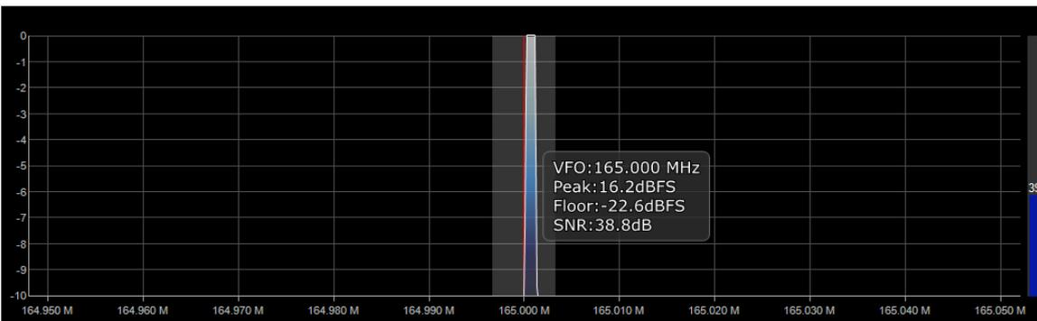
Figure 4. Signal strength when the transmitter facing the left parasitic element shorted by capacitor
