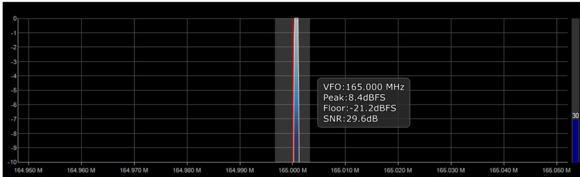
Figure 3. Figure Signal strength when the transmitter facing the parasitic element shorted by inductor
