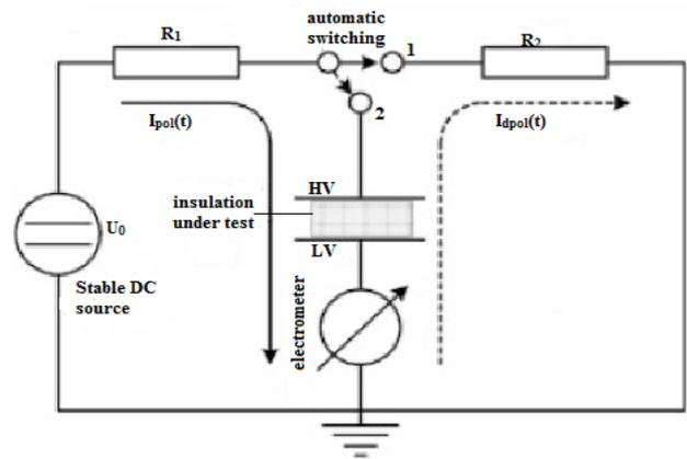
**Figure 4.** Two electrode method for time domain dielectric response dimensions
