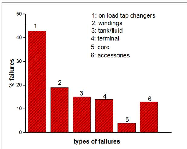
**Figure 3.** Survey results for failures in transformers with on-load tap changers
