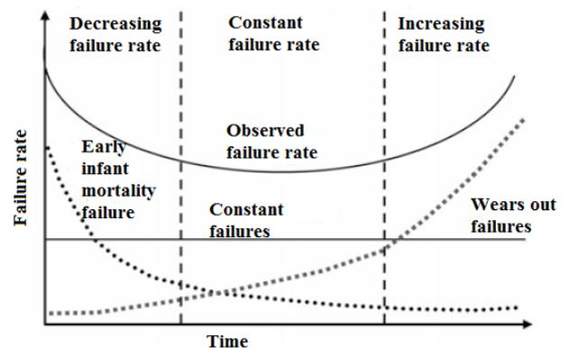
Figure 2. Typical transformer breakdown pattern
