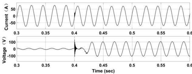
Figure 10. Waveforms of the ES voltage and the noncritical load current with the ES activated
