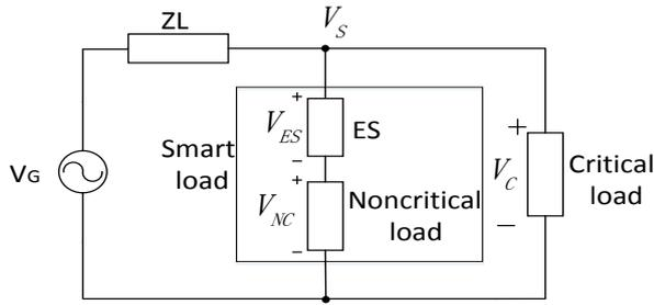
Figure 1. Connecting diagram of ES in the circuit
