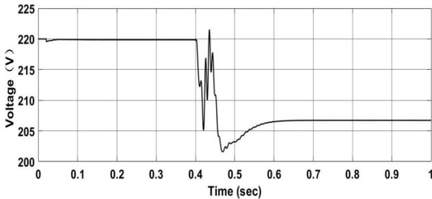
Figure 9. Measured value of the noncritical load voltage  $V_{NC}$  with the ES activated
