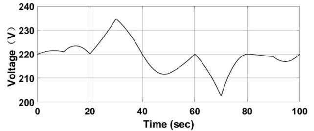
Figure 11. Measured value of the critical load voltage  $V_C$  without ES (in stability test)
