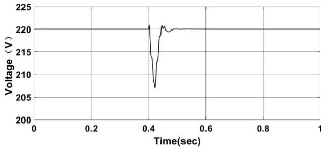
Figure 8. Measured value of the critical load voltage  $V_C$  with the ES activated
