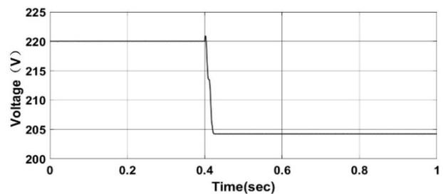
Figure 7. Measured value of the critical load voltage  $V_C$  without the ES
