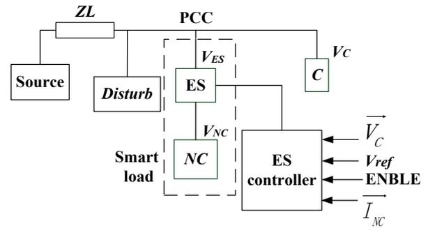
Figure 5. Simplified schematic of voltage stabilizing model using the ES
