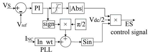
Figure 4. Control block diagram of the ES used in this paper
