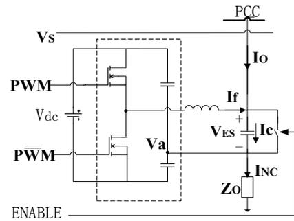
Figure 3. Circuit diagram of the ES
