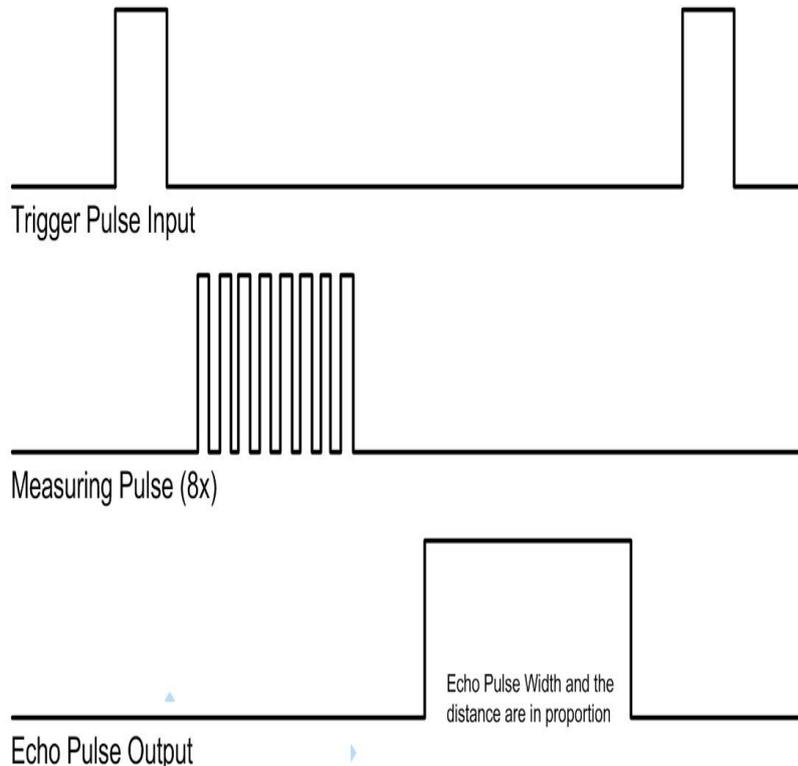
Figure 4. Timing Diagram to explain the working of an Ultrasonic sensor [3]
