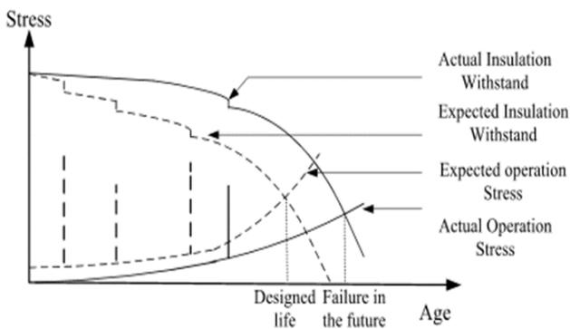
Figure 3. Transformer failure beyond designed life span [18]
