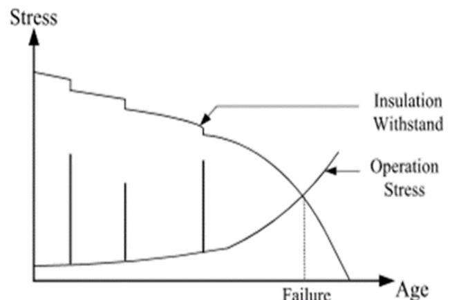
Figure 1. Transformer failure illustration [18]
