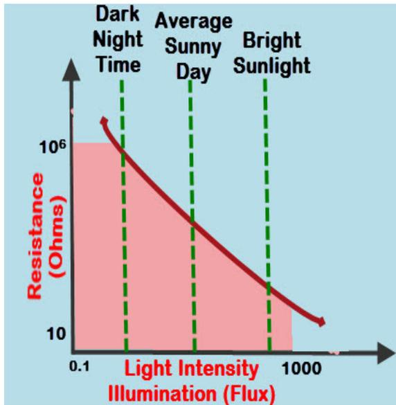
Figure 5. Resistance Vs Light Intensity [6]
