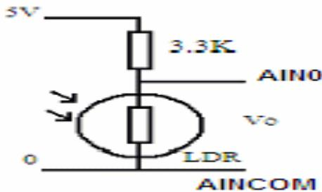
Figure 6. LDR Circuit Diagram [6]
