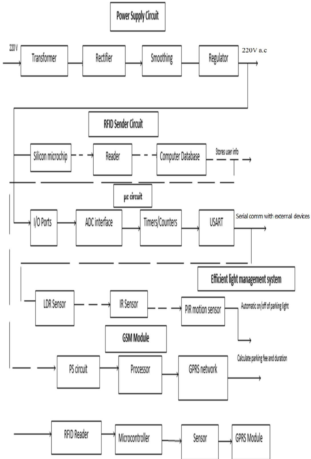
Figure 1. Basic cluster diagram of the entire set-up which has been implemented to achieve the automated power-efficient parking system
