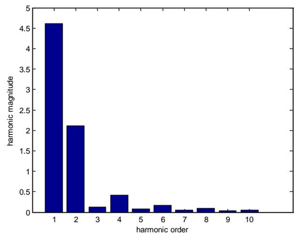
Figure 1. Harmonic spectrum of a rectifier
