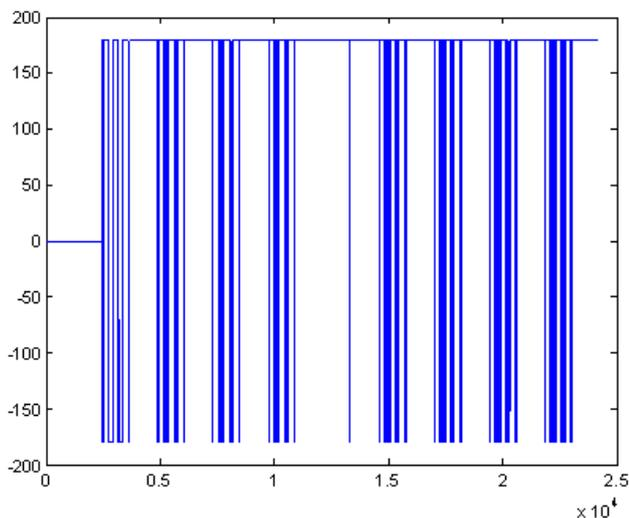
**Figure 2.** Phase behavior of 5<sup>th</sup> harmonic current in a rectifier
