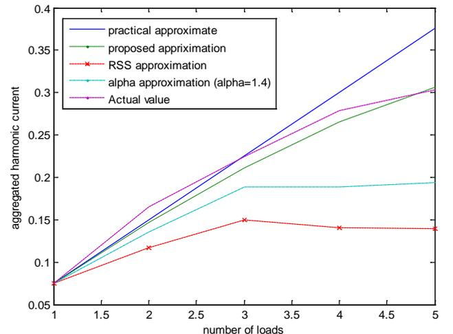
Figure 3. Practical approximations for aggregated 5<sup>th</sup> harmonic current
