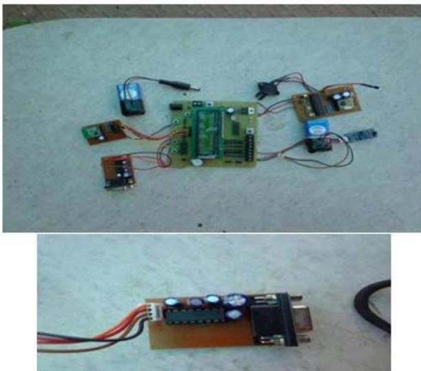
**Figure 3.** Embedded Control Hardware Circuit with serial communicator RS232
