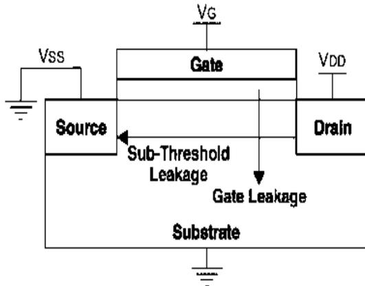
Figure 1. Static CMOS Leakage Power Sources [21]
