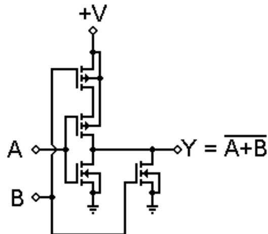
Figure 2. Stack mode approach using 2 input NOR gate [22]
