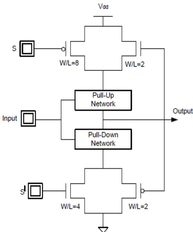
Figure 3. Sleepy Keeper circuit [11,23]
