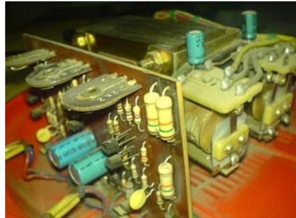
Figure 3.2. a voltage stabilizer using electromechanical relays for switching
