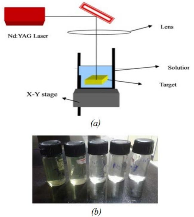
Figure 1. Ablation setup (a) and the solutions containing copper nano particles (b)
