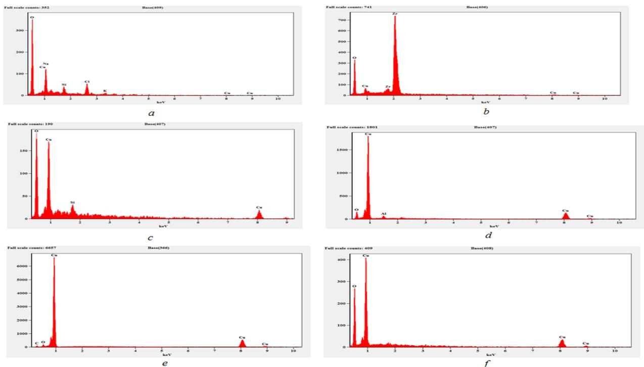
Figure 2. Elemental analysis which shows the percentage of Cu. (a) 30min b) 60 mins c) 90mins (d) 120 and (e) 150 mins of time durations (f) Pure Copper Target
