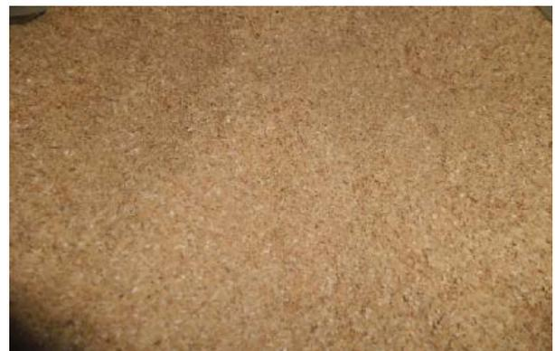
Figure 1. Overview of rice husks to incorporate into fired clay brick
