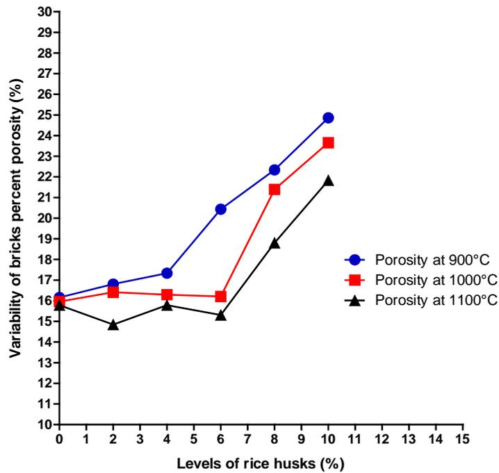
Figure 12. Influence of adjuvant and firing temperature on porometric properties of fired clay bricks
