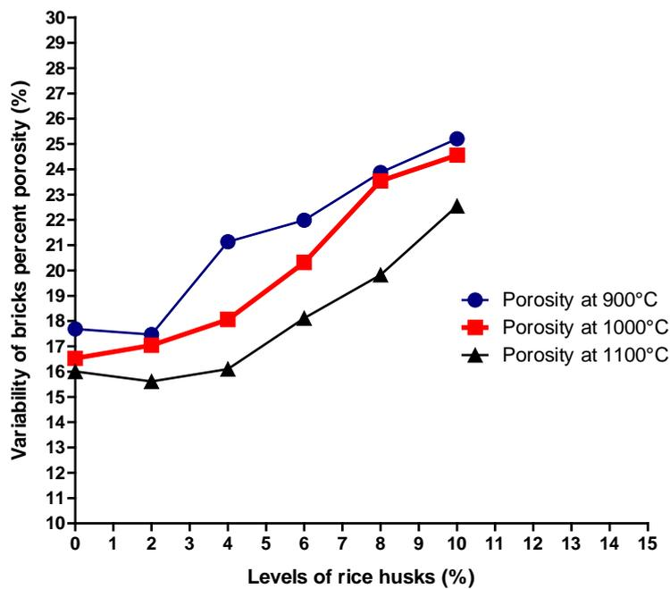
Figure 15. Influence of adjuvant and firing temperature on porometric properties of fired clay bricks
