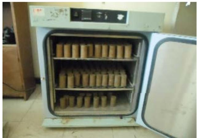
**Figure 9.** Specimens of bricks in an oven set at a temperature of 105°C
