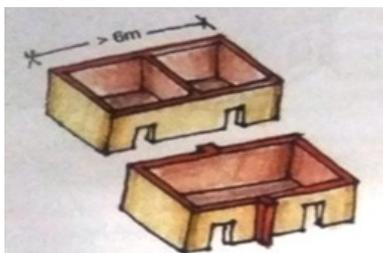
Figure 13. Pilaster of intermediate system to be preferred
