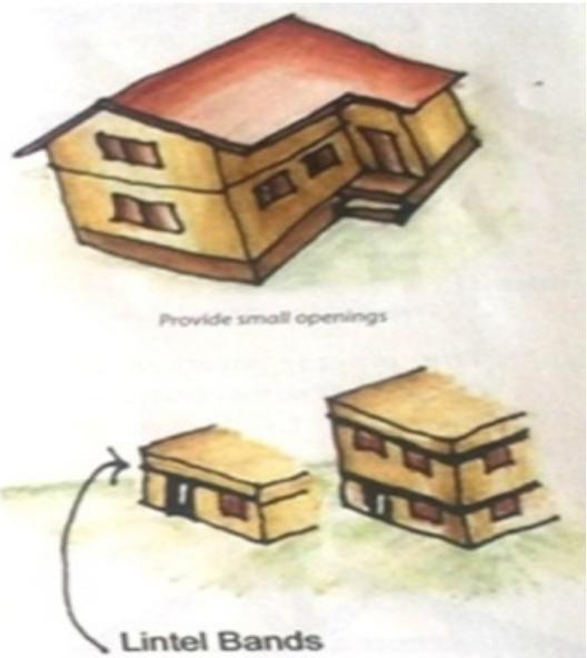
Figure 20. Small openings and lintel bands should be provided
