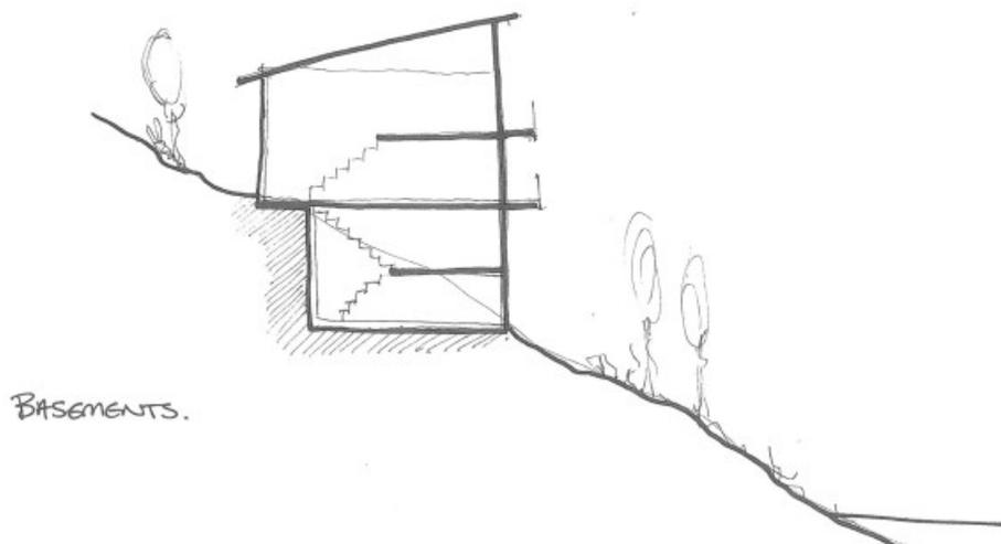
Figure 6. Stepping the ground slope to provide the basement
