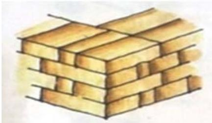
Figure 19. Masonry without continuous vertical joints recommended
