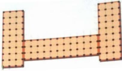
**Figure 23.** The structural grid system should be uniform
