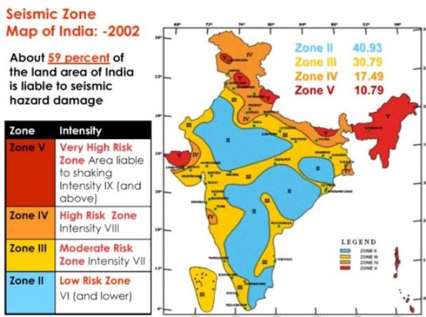
Figure 7. Seismic zones and intensity map of India
