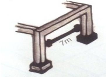
**Figure 24.** The span of beam should not be more than 7m
