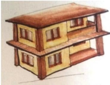
**Figure 25.** Provide opening on same position on all floors
