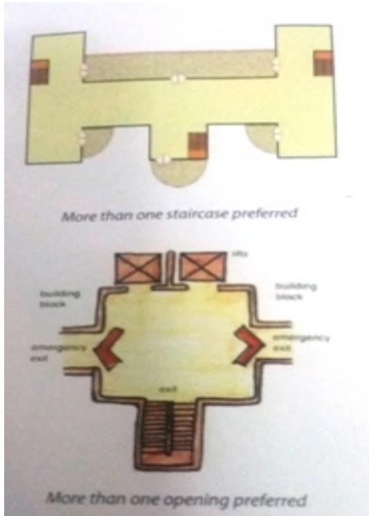
Figure 11. More than one staircase and emergency exit should be provided
