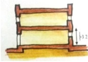
Figure 17. Clear height should not be more than 3.2 m.
