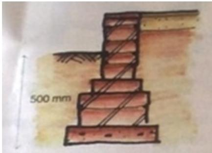
Figure 18. Medium to deep foundations should be preferred.
