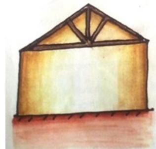
Figure 22. Gable band for gable wall should be provided.
