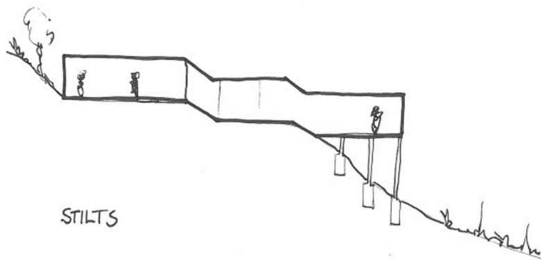
Figure 5. Building on stilts addresses the construction on steeply slope site.
