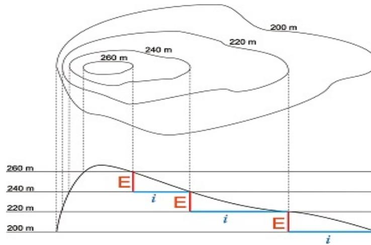
Figure 2. Contour map showing lines joining points of equal elevation on a surface
