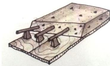
**Figure 26.** Proper reinforcement with non-corroding spacers should be provided
