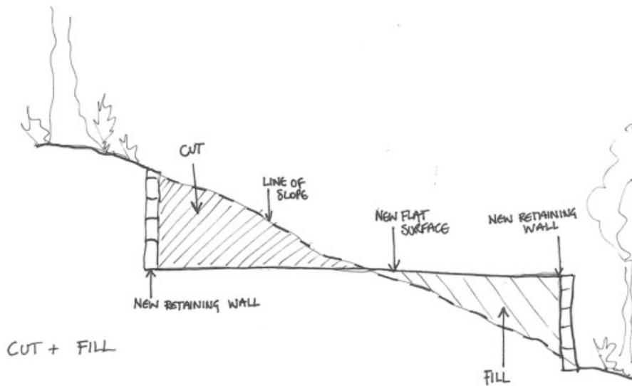
Figure 4. Cut and fill technique for developing flat surface.
