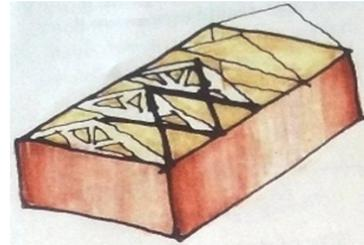
Figure 21. Bracing of roof truss should be provided.
