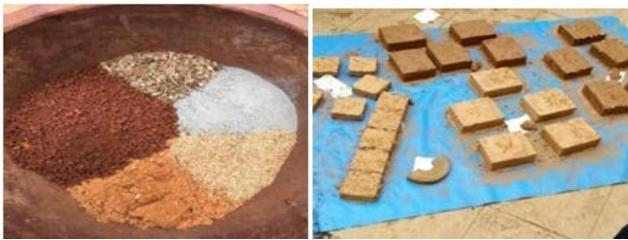
Figure 3. Example of brick formulation (laterite, typha, rice hull and cement)
