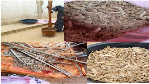
Figure 2. Preparation of Typha and rice hull samples
