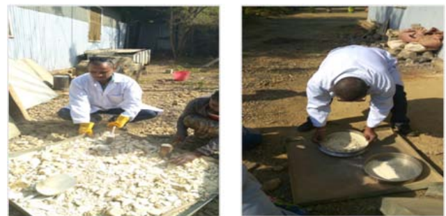
Figure 3. Preparation for Lab Test of Physical Property of Natural Subbase Material (Source: Photos taken during the laboratory works)
