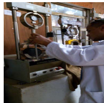
Figure 5. Marshall Stability Test (Source: Photo taken during the experiment)
