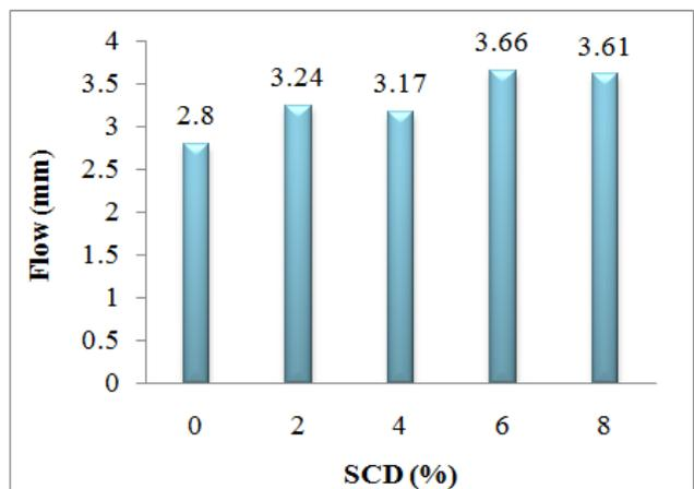
Figure 8. Asphalt Mix Flow – Filler Content Relationship
