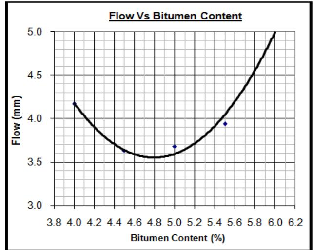
Figure 6. Flow Vs. Bitumen Content
