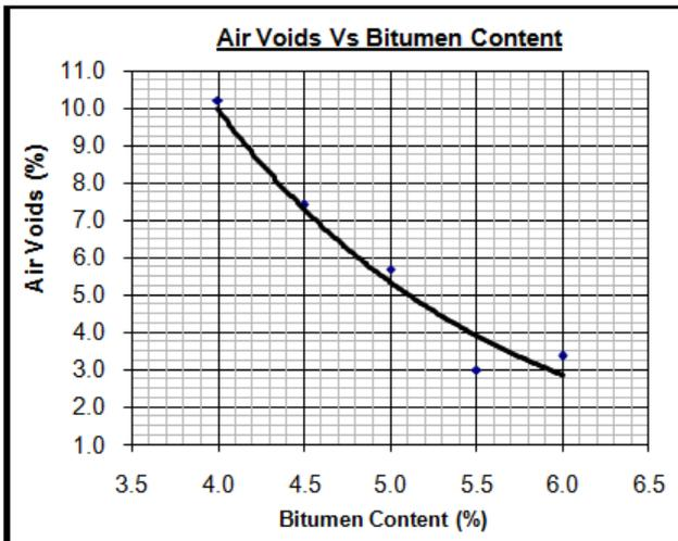
Figure 5. Air Void Vs. Bitumen Content
