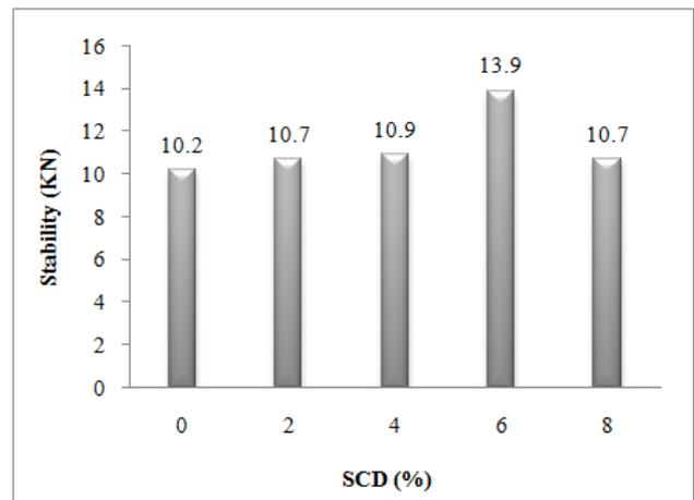
Figure 7. Asphalt Mix Stability – SCD Filler Content Relationship
