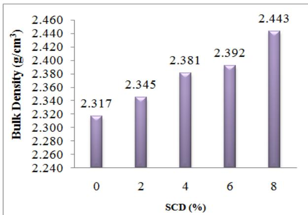
Figure 9. Asphalt Mix Bulk Density – Filler Content Relationship
