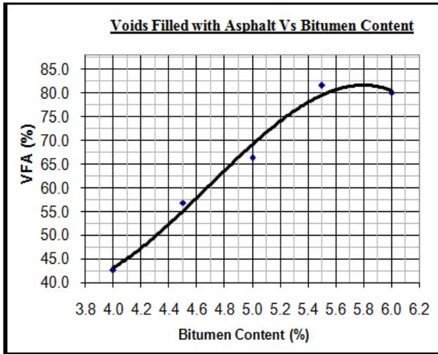
Figure 4. VFA Vs. Bitumen Content
