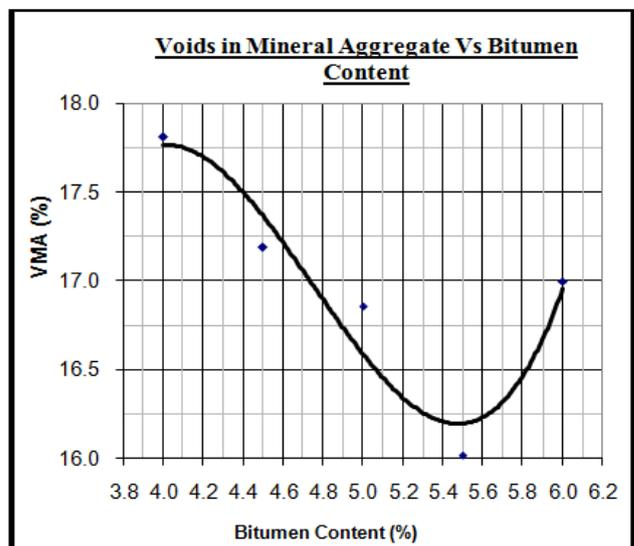
Figure 3. VMA Vs. Bitumen Content
