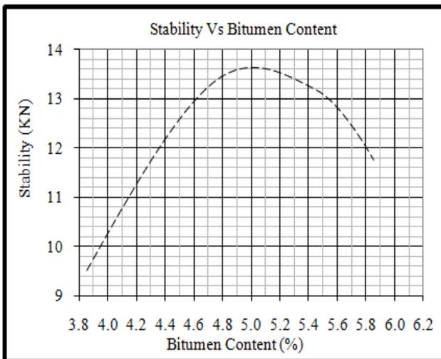
Figure 1. Stability Vs. Bitumen Content
