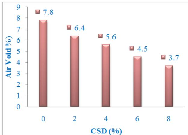
Figure 10. Asphalt Mix Air Voids – Filler Content Relationship
