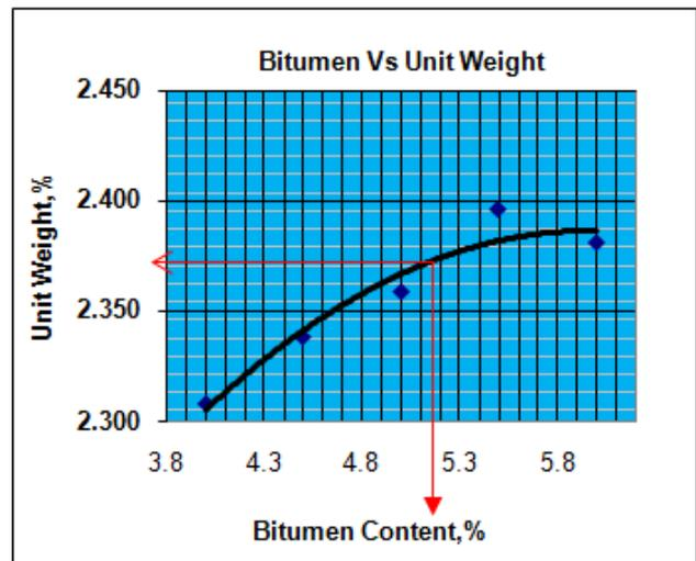
Figure 2. Unit Weight Vs. Bitumen Content
