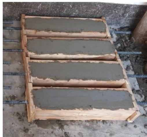
Figure 2. Preparation of Prismatic sample
