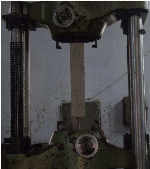
Figure 3. Test Setup for axial tension test of RC members
