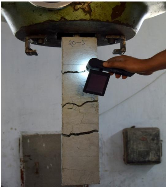
Figure 4. Crack measurement with microscope
