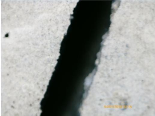
Figure 6. Image of crack width by microscope
