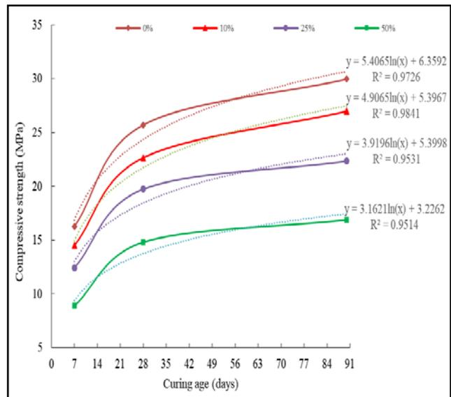
Figure 9. Development of compressive strength under 90 days water curing
