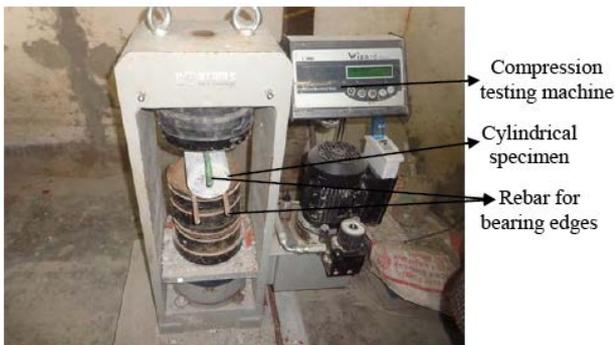
Figure 6. Test set-up for splitting tensile strength test
