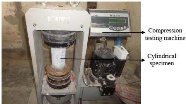
Figure 5. Placement of cylindrical specimen for compressive strength test
