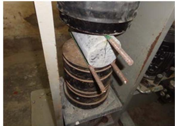
(a) Splitting cracks observed during tensile loading
