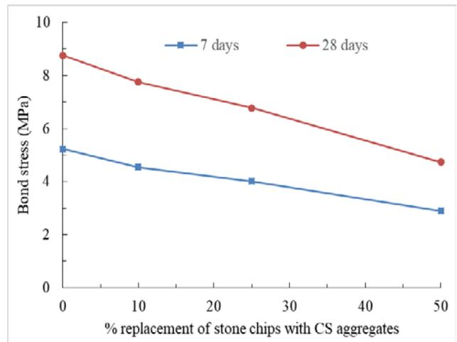
Figure 13. Bond stress of normal concrete and concrete containing different percentage of coconut shell aggregates at 7 and 28 days age
