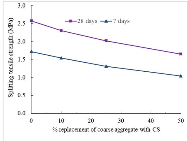
Figure 11. Variation of tensile strength with percentage replacement of coarse aggregates by crushed coconut shells at 7 and 28 curing days
