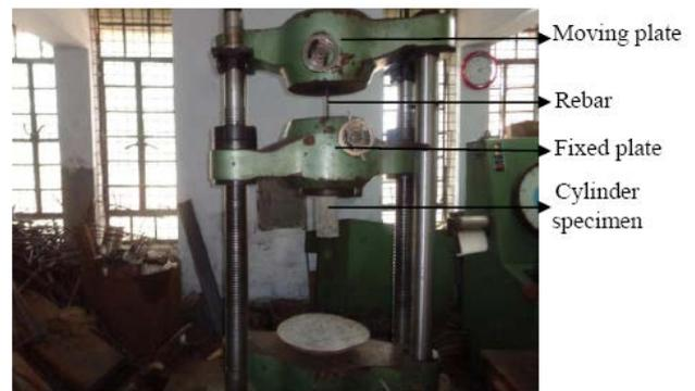
Figure 7. Direct pullout test set-up for the determination of bond stress-slip behavior
