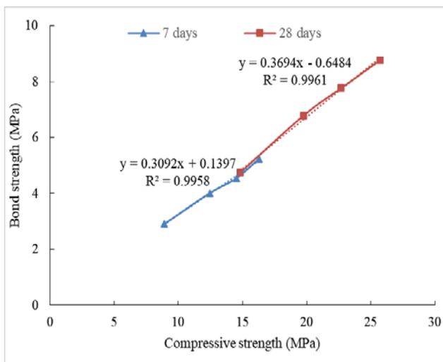
**Figure 15.** Relationship between bond strength and compressive strength
