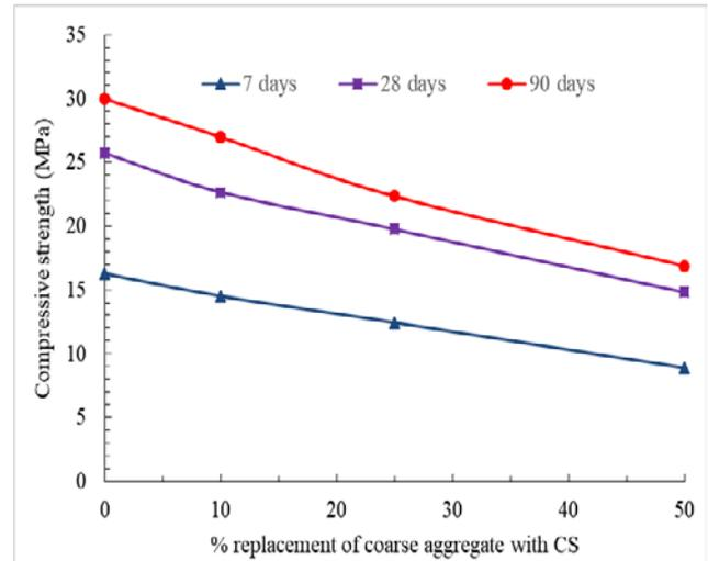
Figure 8. Comparison of compressive strength of concrete with percentage replacement of coarse aggregates by crushed coconut shells at 7, 28 and 90 curing days.
