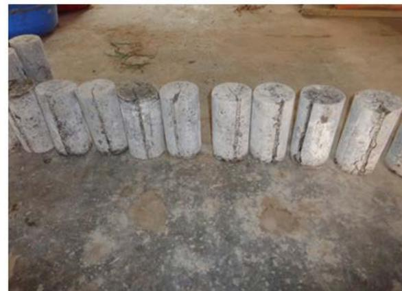
(b) Observation of splitting cracks after testing
