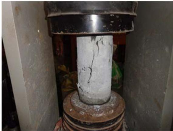
(a) Observed cracks during testing
