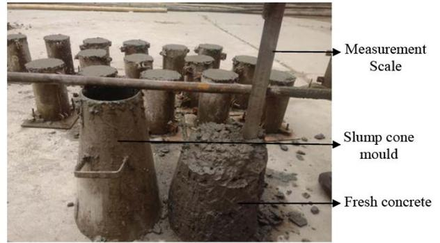
Figure 2. Slump cone test to measure the workability of concrete
