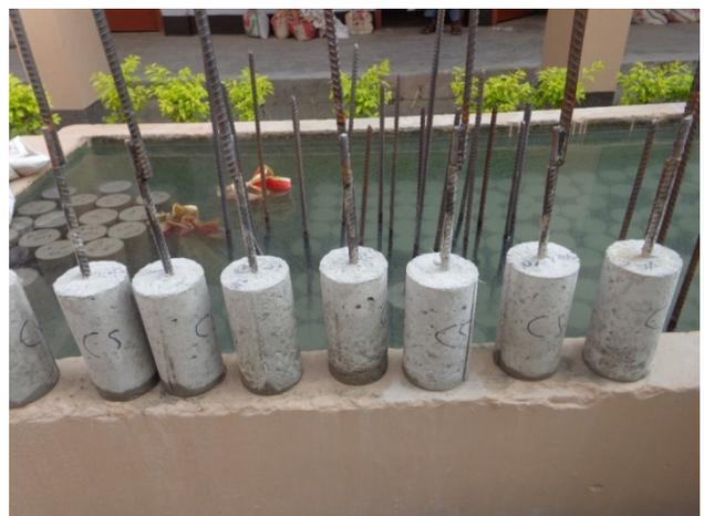
Figure 4. Preparation of test specimens to evaluate bond properties
