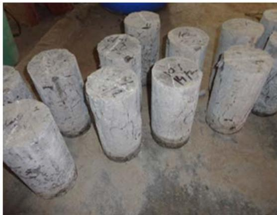
(b) Observation of cracks after testing
