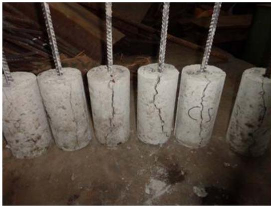
(b) After bond test of specimens
