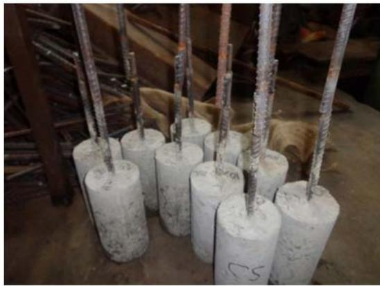
(a) Before bond test of specimens
