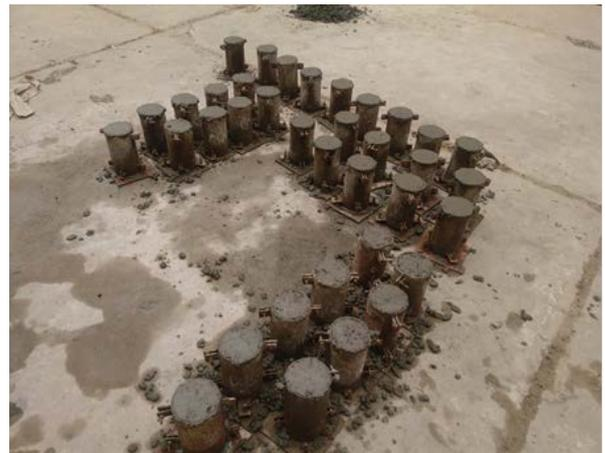
Figure 3. Preparation of cylindrical specimens for compression and tension testing
