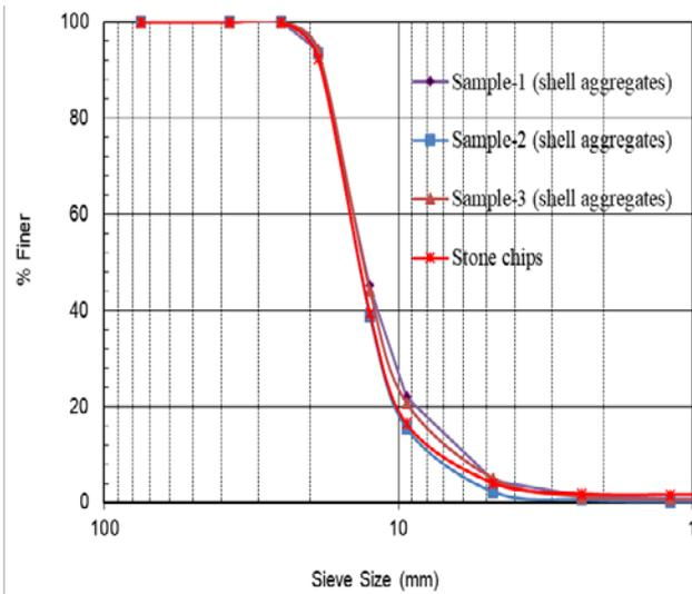
Figure 1. Grain size curves for stone chips and crushed coconut shell aggregates
