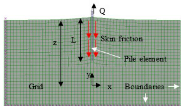
Figure 2. Generated mesh, boundary conditions and the pile element
