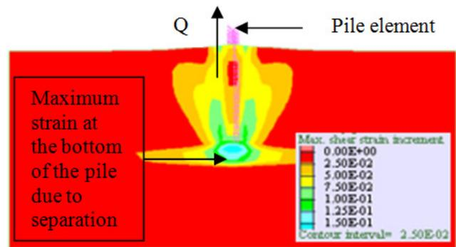
Figure 7. Maximum shear strain increment around the pile element
