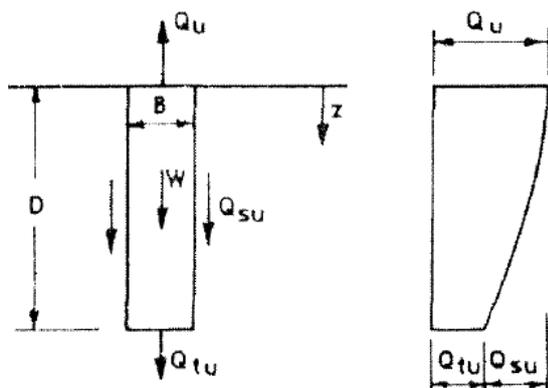
Figure 1. Uplift capacity function and the failure pattern by Kulhawy
