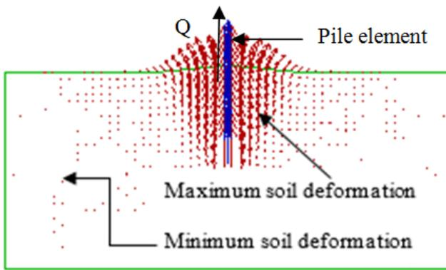
Figure 4. Ground movements during axial loading
