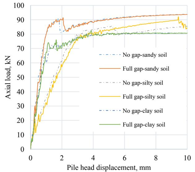
Figure 10. Effects of the gap on the ultimate axial load
