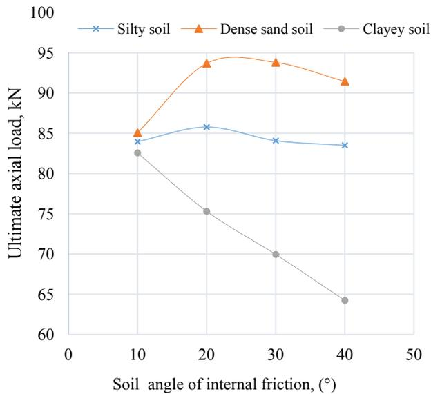
Figure 9. Influence of the angle of internal friction of the soil
