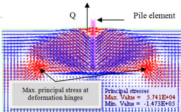
Figure 6. Effective Principal stress tensor distribution on axial loading
