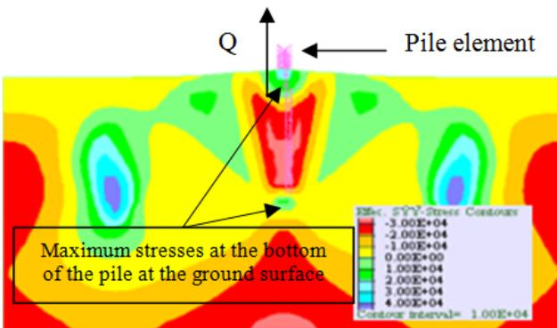
Figure 5. Contour zone for effective stress distribution on the grid
