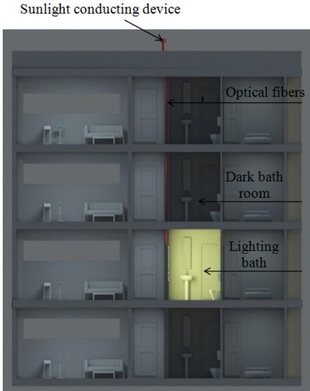
Figure 3. Sunlight transferring system to dark spots by optical fibers
