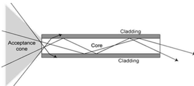
Figure 1. Light conduction in an optical fiber [14]
