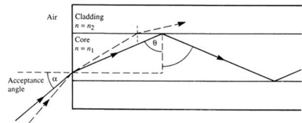
Figure 2. Refraction of light in an optical fiber [18]:  $n_2$  is the refractive index of the cladding,  $n_1$  is the refractive index of the core,  $\alpha$  is the acceptance angle of the fiber,  $\theta$  is the angle of incidence
