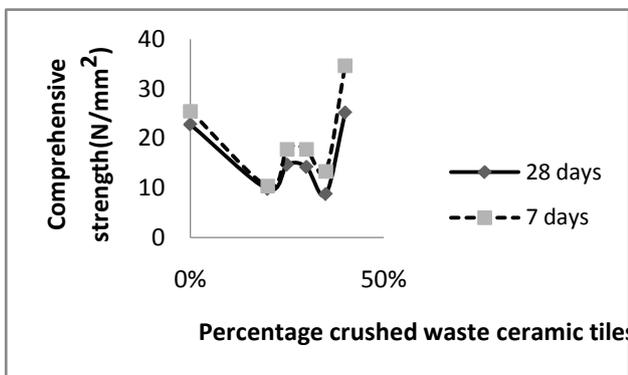
Figure 1. Plot of compressive strength versus crushed waste ceramic tile
