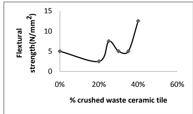
Figure 2. Plot of flexural strength versus crushed waste ceramic tile
