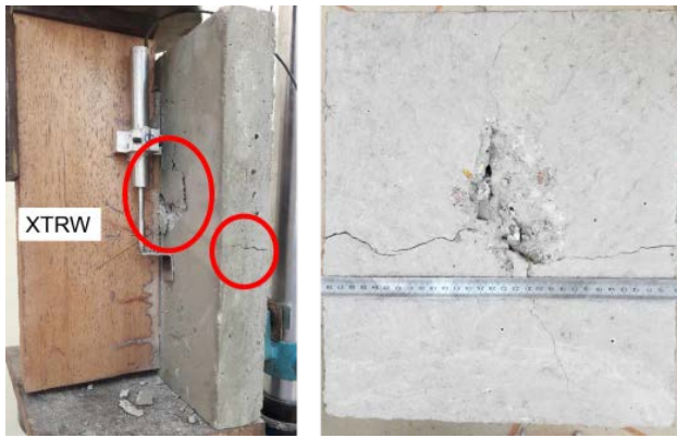
Figure 8. Cracking in concrete slab (XTRW - cross-threaded rebar connection without interlayer)
