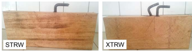
Figure 2. Threaded Rebars after Screwing into the Timber
