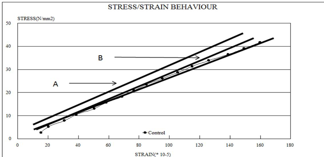
**Figure 1.** Idealized Stress – Strain Curves: A – Concrete with 25% rice husk ash, B – Concrete with 50% rice husk ash
