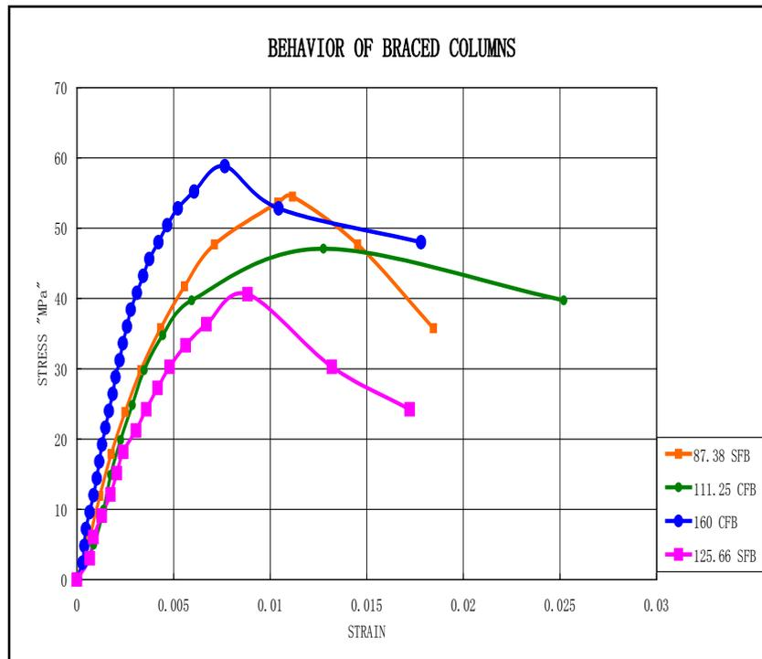
Figure 4. Stress – strain curve of braced columns
