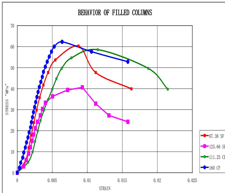
Figure 3. Stress – strain curve of filled columns
