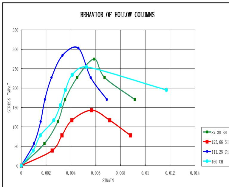
Figure 2. Stress – strain curve of hollow columns
