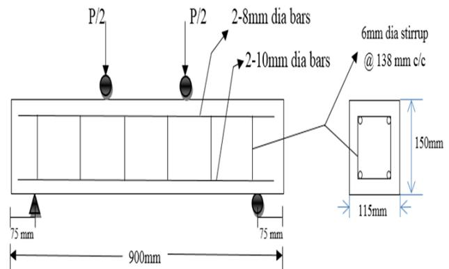
Figure 1. Geometry and sectional details of test specimen
