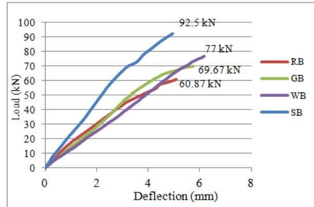
Figure 6. Load-Deflection curve of different tested beam sample
