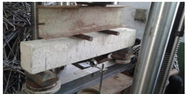
Figure 2. Reference beam (RB) under testing
