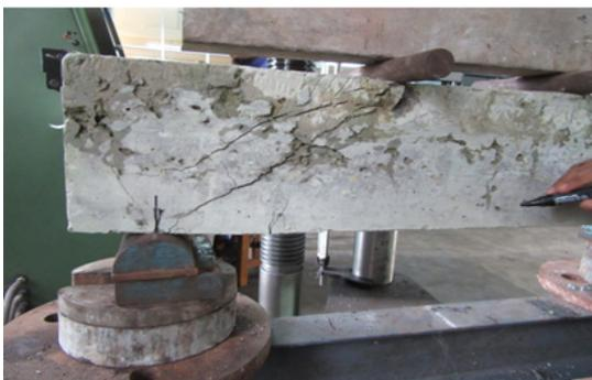
Figure 5. Testing of beam with additional steel bars and its failure pattern
