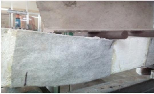
Figure 3. Testing of beams strengthened with geo-textile
