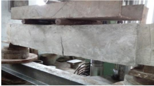
Figure 4. Beam strengthened with wire mesh under testing with failure pattern
