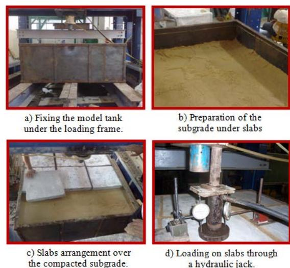
**Figure 1.** Stages of the Conducted Loading Test on Model Slabs
