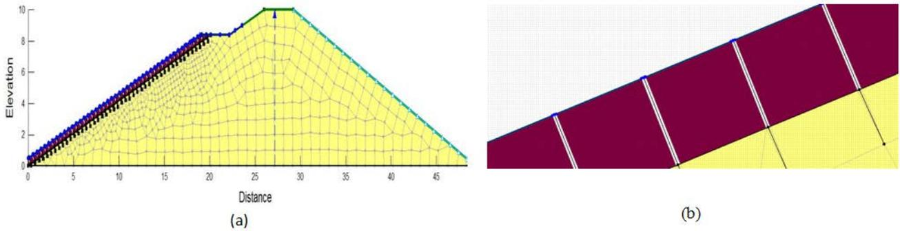
Figure 7. (a) Embankment model in SEEP/W software (with CC Block) (b) Enlarged view of CC Blocks
