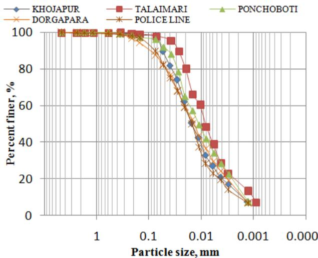
Figure 3. Particle size distribution curve for different sections
