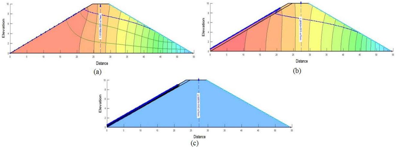
Figure 9. Seepage analysis considering (a) without CC Block (b) with CC Block (c) joint sealed
