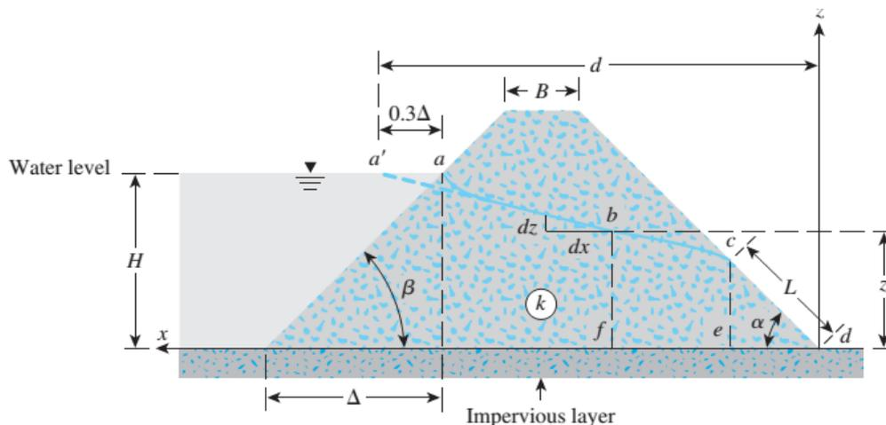
Figure 5. Flow through an embankment constructed over an impervious base (Principles of Geotechnical Engineering, BM Das)
