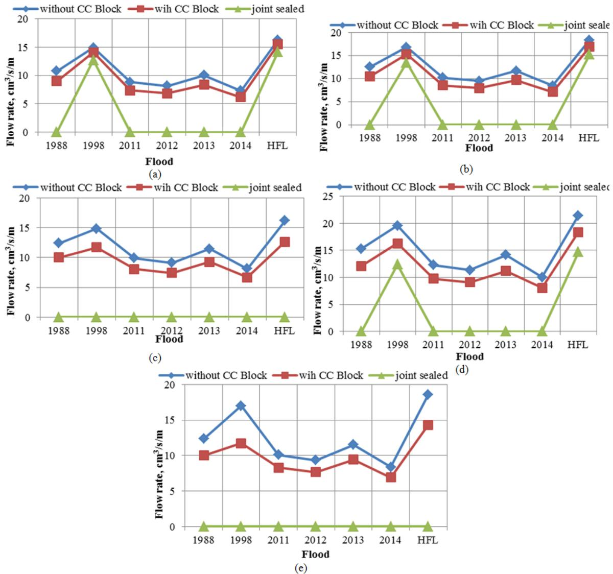
Figure 11. Flow rate through embankment at (a) Khojapur (b) Talaimari (c) Ponchoboti (d) Dorgapara (e) Police Line section
