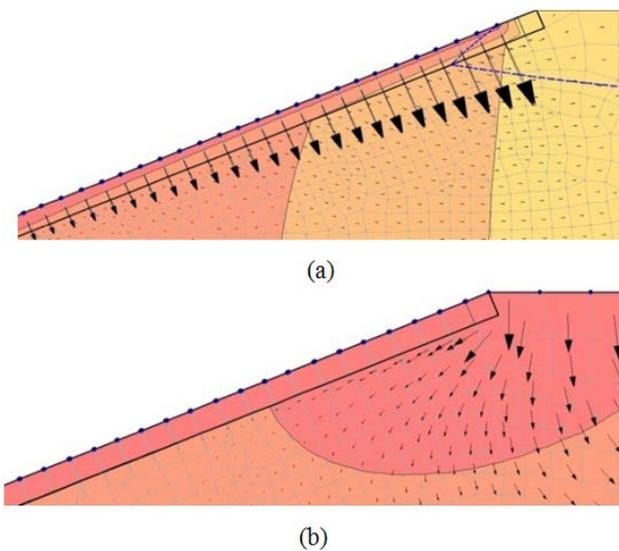
Figure 10. (a) Flow of water through the joints between the CC Blocks (b) No flow of water through the joints between CC Blocks
