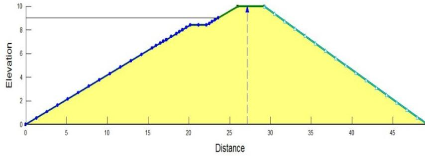
Figure 6. Embankment model in SEEP/W software (without CC Block)
