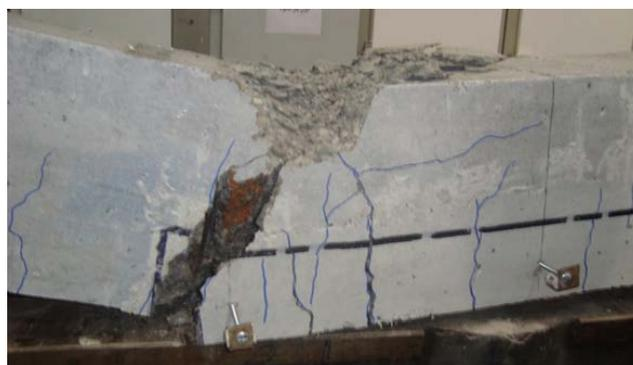
Figure 13. Ultimate cracking and failure of beam F5\
