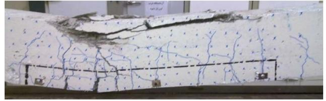
Figure 14. The final crack pattern and failure of beam F4
