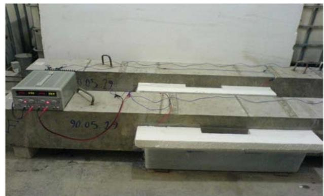
**Figure 4.** Photo of setup for accelerated corrosion test
