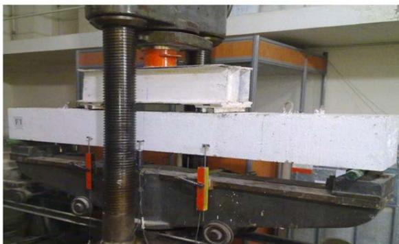
Figure 7. Flexural PT beam test set
