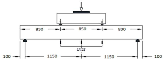
Figure 8. Flexural load test details (in mm)
