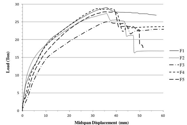
**Figure 11.** Comparison of load-displacement response of PT beams
