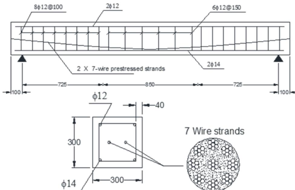
Figure 2. Geometry of the PT beams and reinforcement layout (mm)
