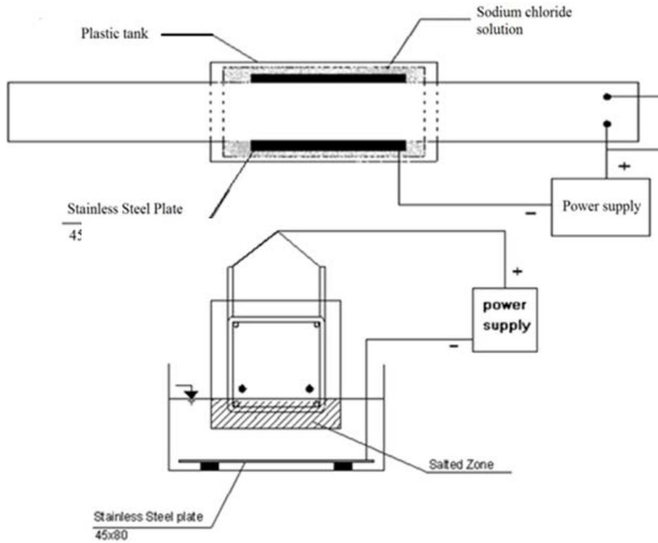
Figure 5. Details of accelerated corrosion test setup
