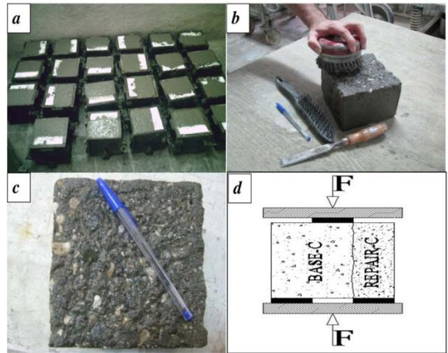
Figure 1. Photos and details of the Bi-Surface shear test procedure
