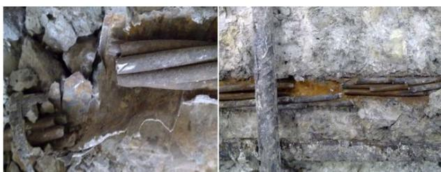
Figure 12. Right: Rupture of strands for F3 beams, Left: Other specimens
