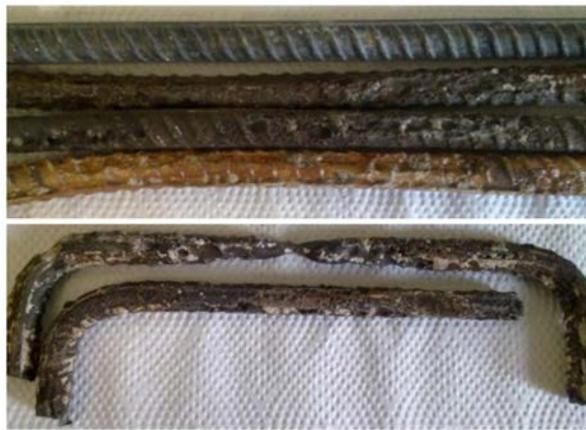
**Figure 9.** Corroded reinforcement, extracted from specimens after conducting all tests. Top: Longitudinal deformed rebars. Bottom: shear deformed rebars
