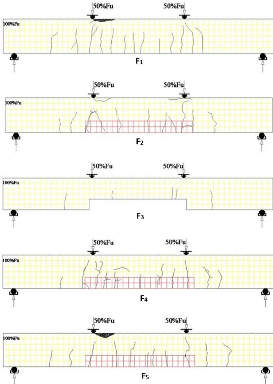
Figure 15. Schematic crack patterns for PT beams at ultimate loads From the top: F1, F2, F3, F4, F5
