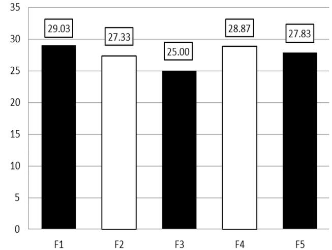
**Figure 10.** Ultimate loads of PT beams (tons)
