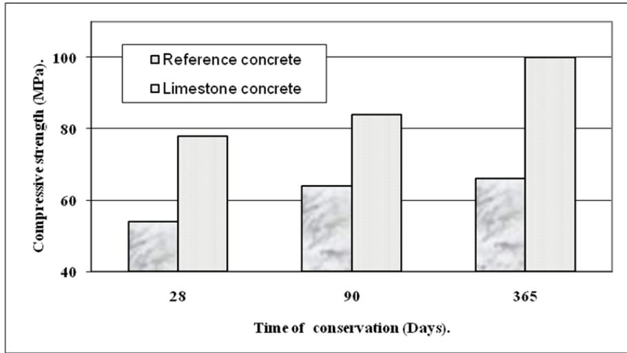
Figure 6. Influence of curing time on the specimen compressive strength
