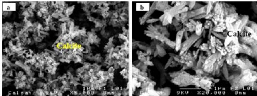
Figure 4. Scanning electron micrograph of ground limestone
