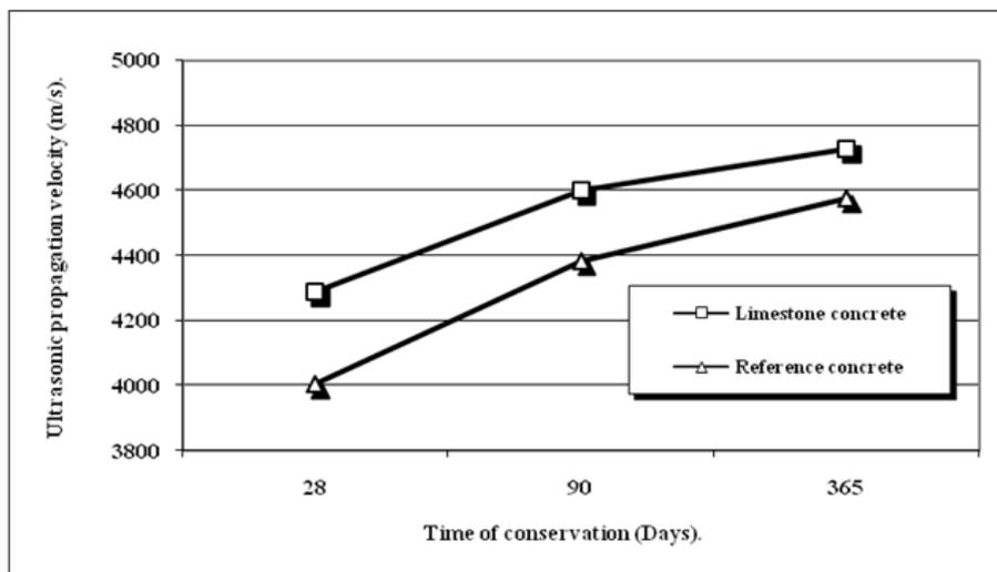
Figure 9. Influence of curing time on sound wave velocity through the elaborated concretes
