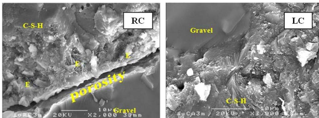
Figure 13. Scanning electron micrograph of the interfacial transition zone of different concrete specimens
