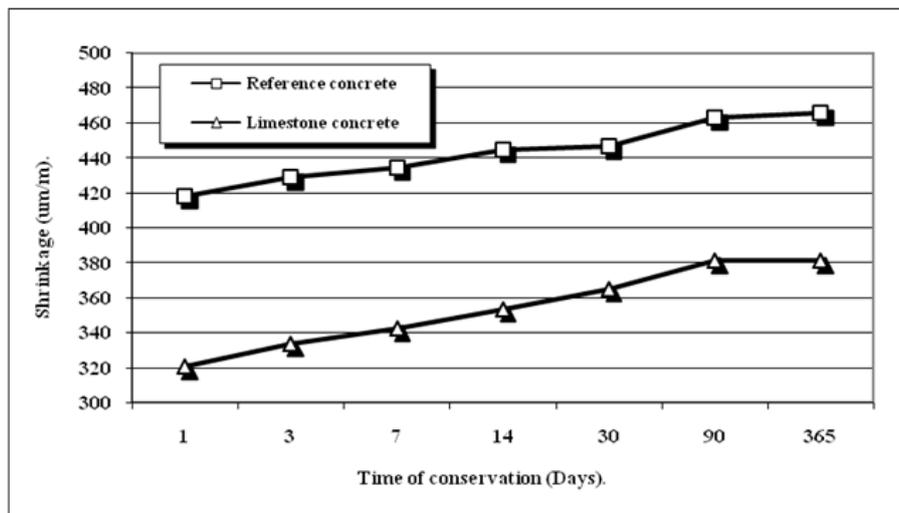
Figure 10. Influence of curing time on shrinkage of the different concretes
