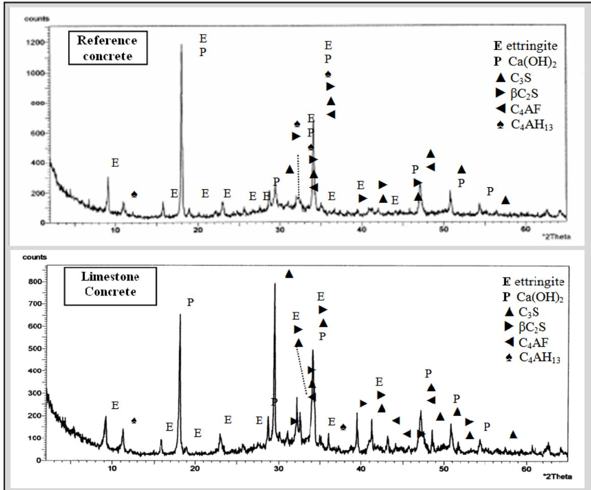
Figure 14. X-ray diffraction analysis of concrete specimens after 365 days of hardening
