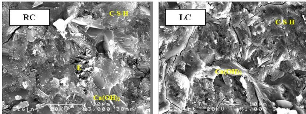
Figure 12. Scanning electron micrograph of different concrete specimen microstructure
