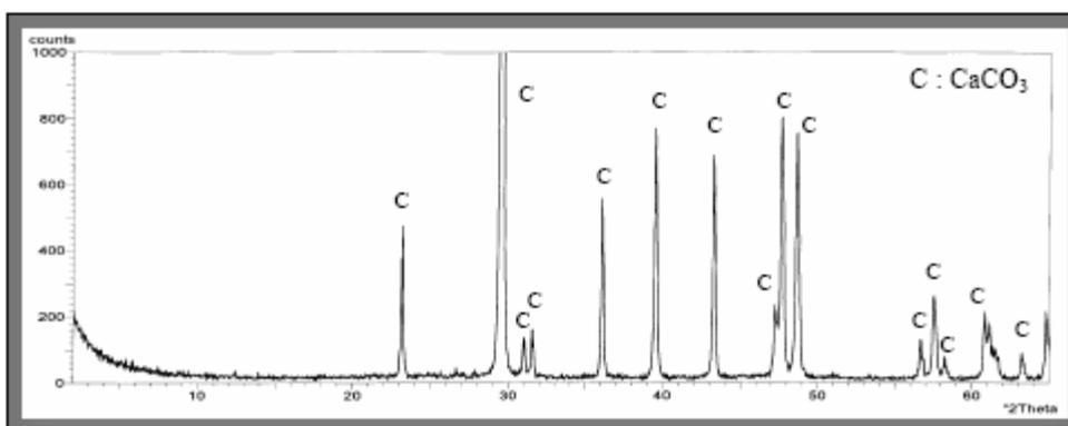
Figure 3. X-ray diffraction analysis of limestone (Cu  $K_\alpha$  filtered)
