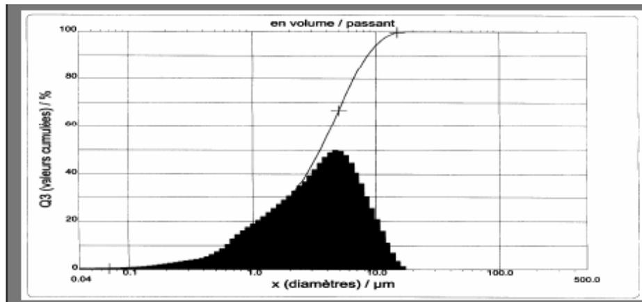
Figure 5. Grading distribution of limestone
