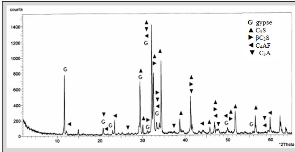
Figure 1. X-ray diffraction analysis of anhydrous cement CEM I 52,5 ( $\lambda$ Cu  $k_\alpha$  filtre Ni)
