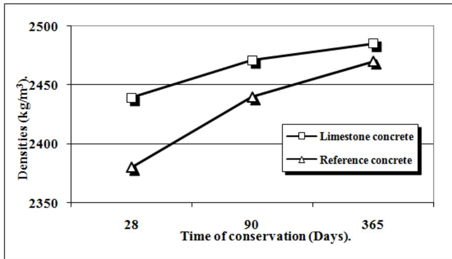
Figure 8. Influence of curing time on concrete density
