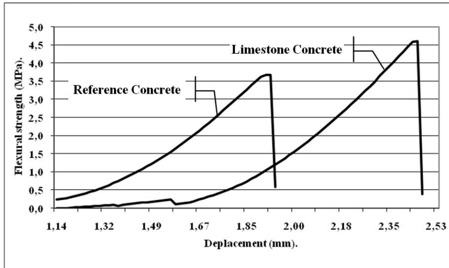
Figure 7. Flexural stress – displacement curves evolution after 3 months hardening
