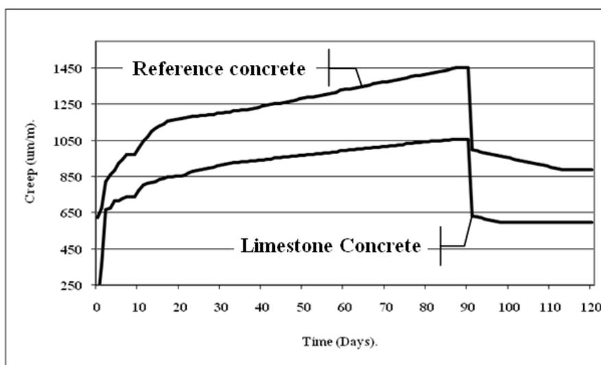
Figure 11. Creep evolution of the different concretes
