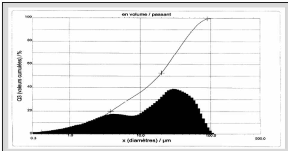
Figure 2. Grading distribution of anhydrous cement CEM I 52.5
