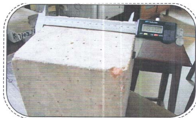
Plate 1. Shrinkage Measurement with Digital Veneer Calipers
