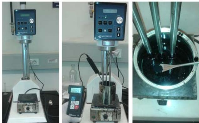
Figure 7. Mixing Asphalt with Carbon Nanotubes using High Shear Mixer
