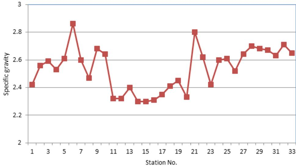
Figure 5. Specific gravity test results at different stations within Koya city
