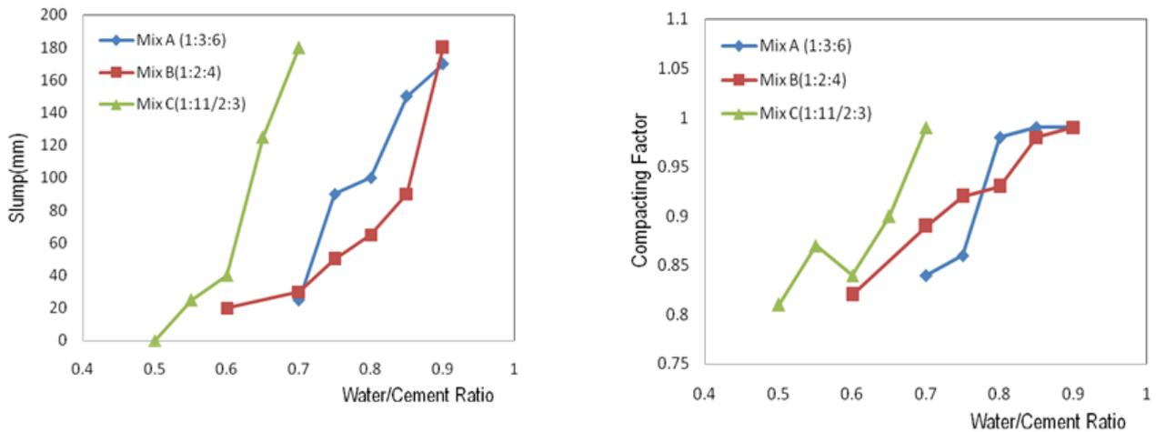
Figure 2. Variation of slump and compacting factor with water/cement ratio and
