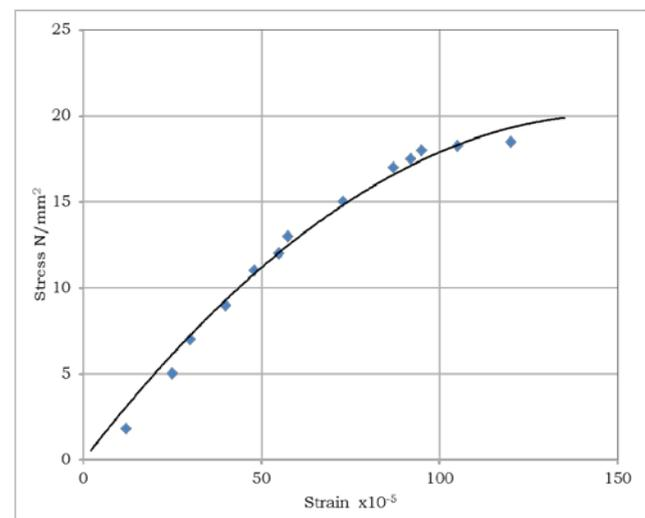
**Figure 5.** Stress-Strain Relationship of Laterite Rock Concrete
