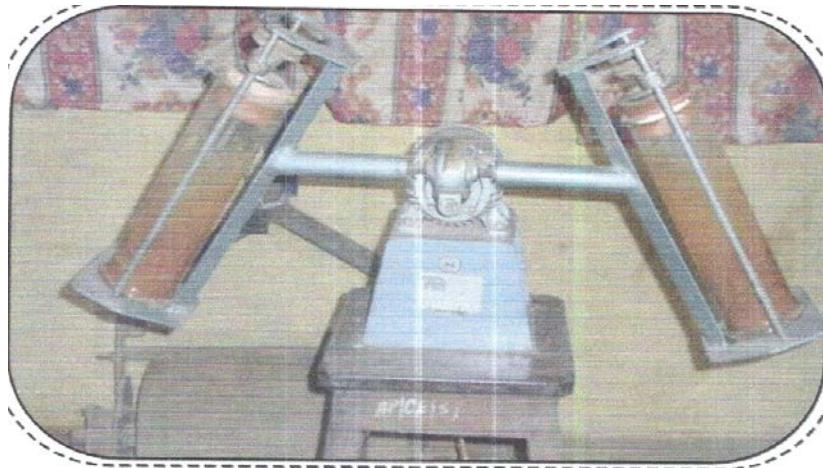
Plate 1. Mechanical shaker for Gs test
