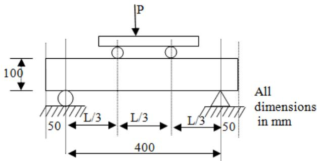
Figure 1. Third point loaded system
