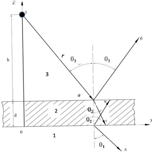
**Figure 1.** Seismic wave passing through fissure from blasting of vertical borehole charge
