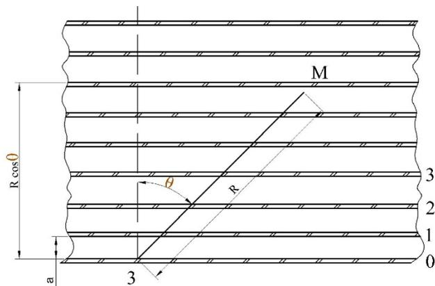
Figure 2. The scheme of seismic waves distribution in anisotropic medium with parallel fracture system
