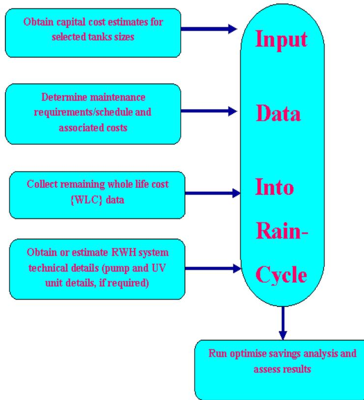
Figure 5. Determining cost savings of tanks and choosing optimum size
