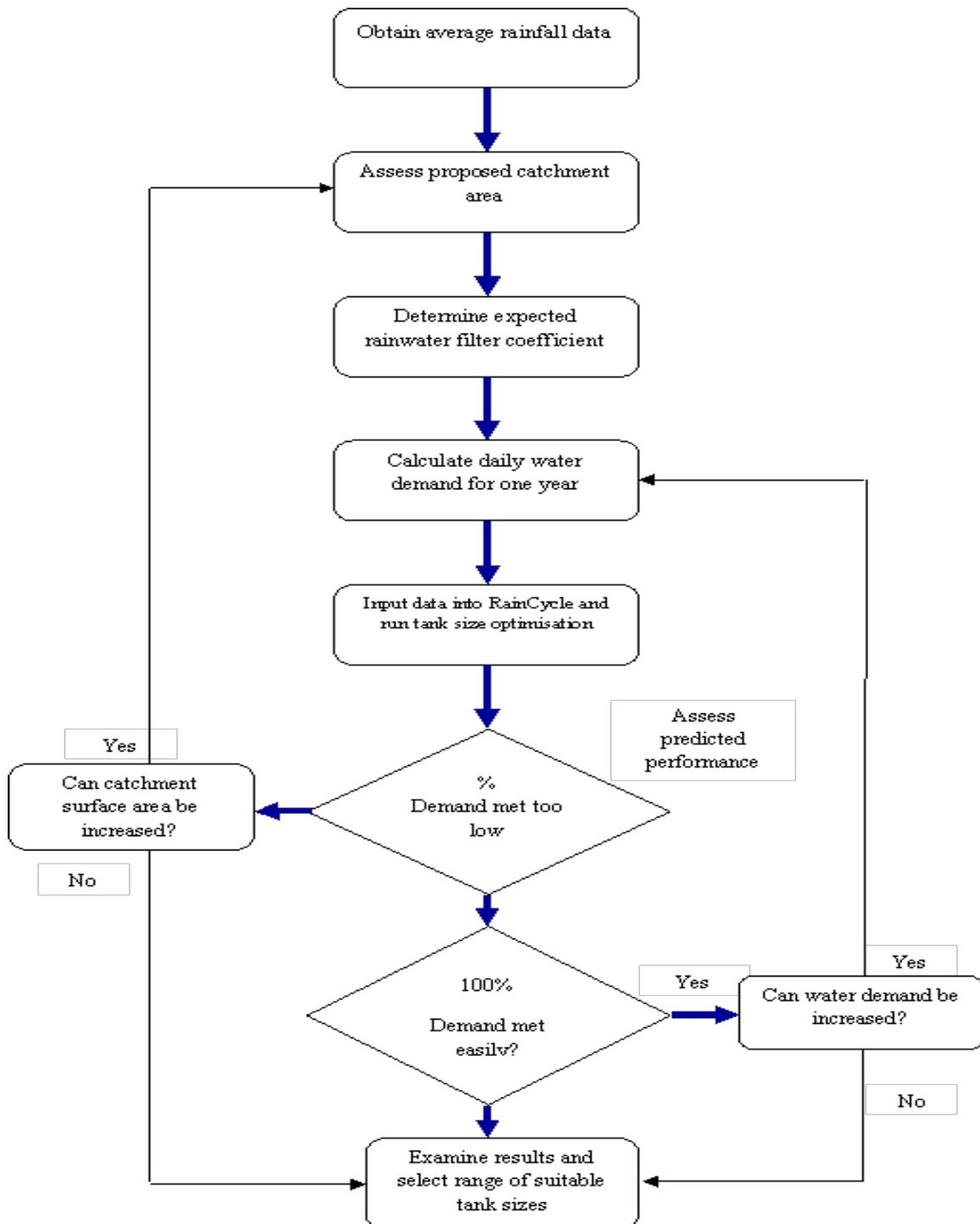
Figure 4. Determining range of suitable tank sizes
