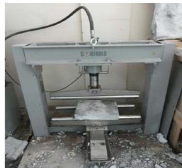
**Figure 3.** Rupture test apparatus
