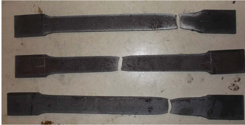
Figure 9. Three failed specimens under tensile loading
