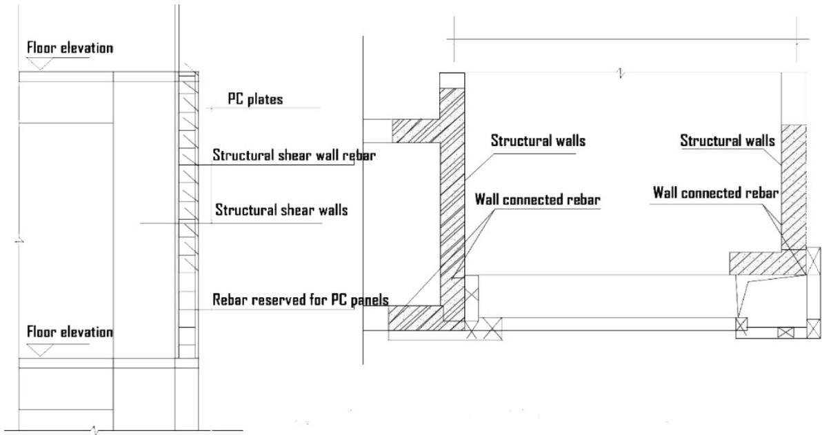
Figure 10. Typical reinforcement installation node
