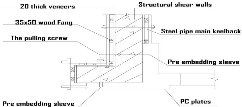
Figure 11. Typical formwork installation
