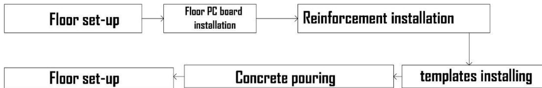
Figure 1. Main construction flow chart of prefabricated buildings
