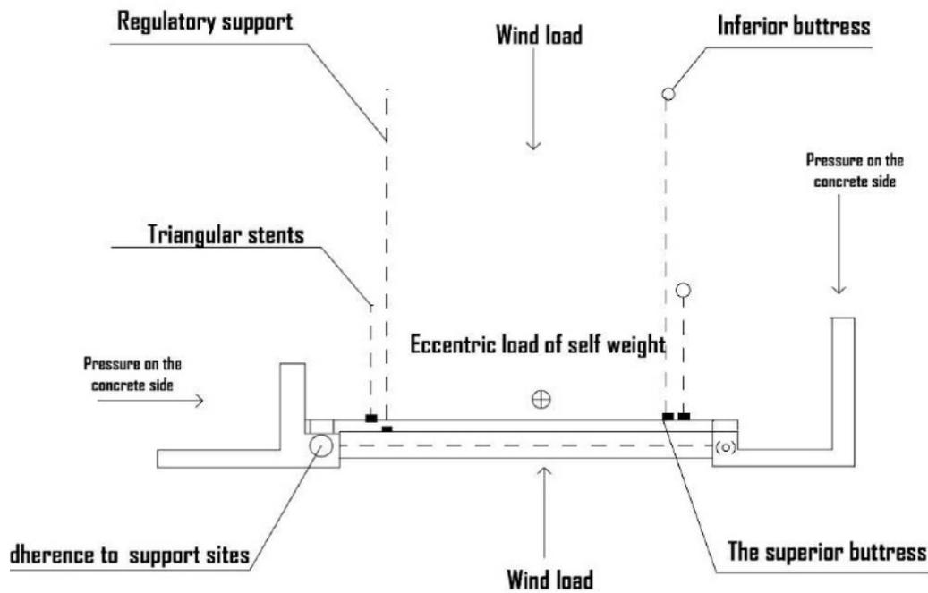
Figure 3. Stress analysis of PC board under temporary support
