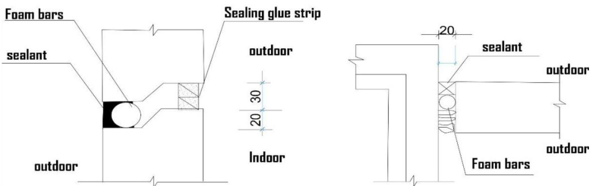
Figure 12. Waterproof of PC board joint
