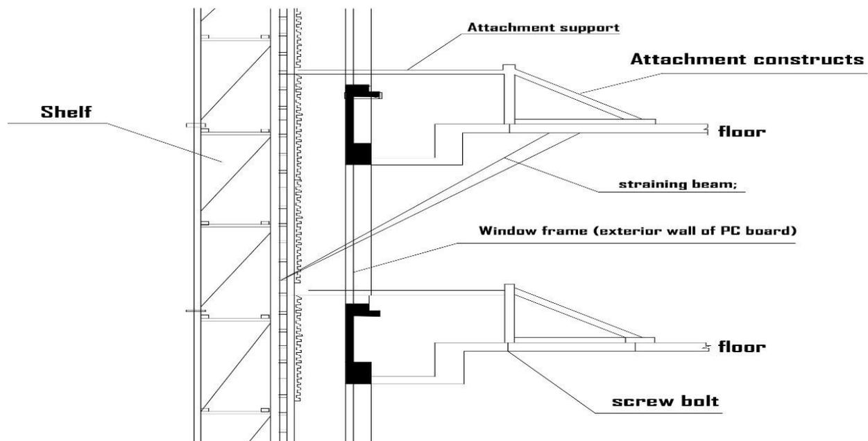
Figure 9. Attachment and installation of climbing frame
