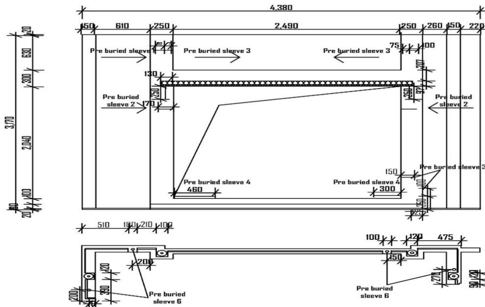
Figure 2. Typical detailed drawing of PC board
