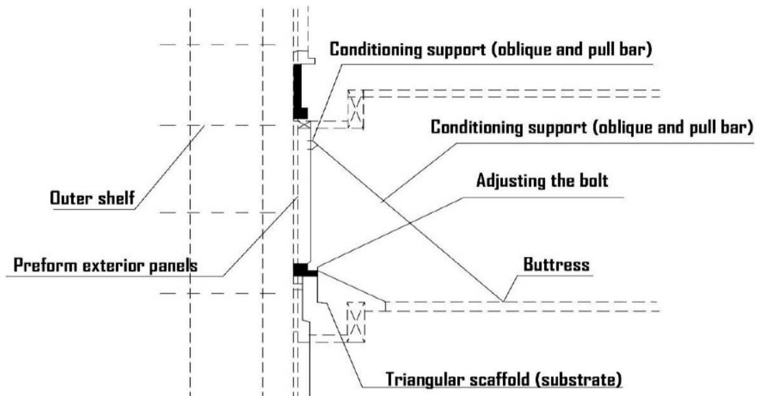
Figure 4. Diagram of the temporary support system
