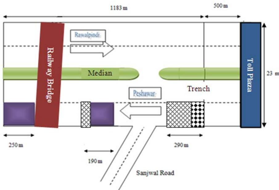
Figure 2. Site layout and testing plan of selected National Highway (N-5) portion
