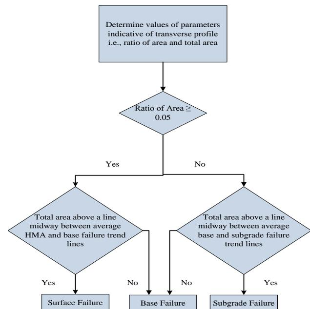
Figure 1. Illustration of procedure for failed layer prediction [13,14]
