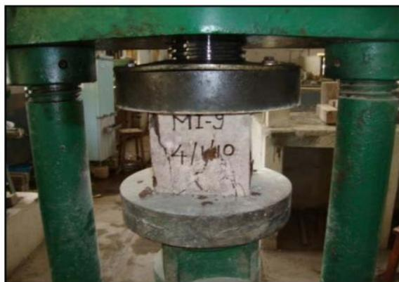
Figure 3. Cube compression test
