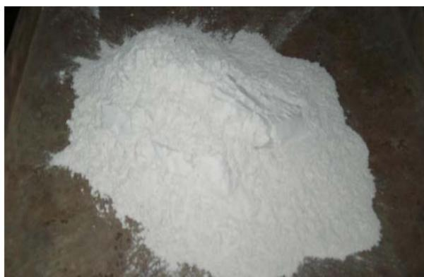
Figure 1. Ceramic waste in dust form
