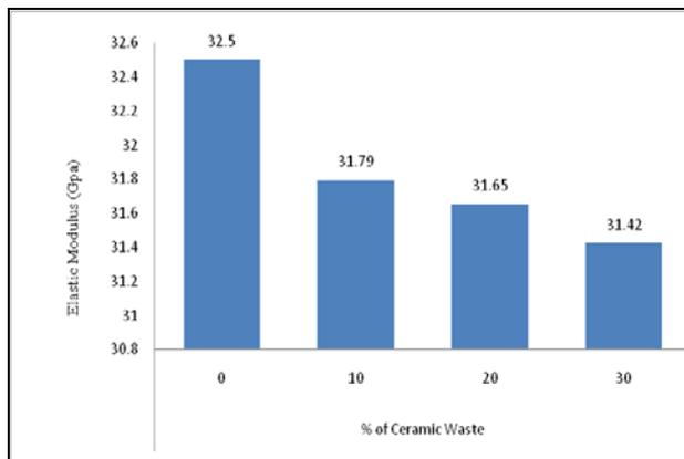
Figure 8. Elastic Modulus of ceramic based concrete
