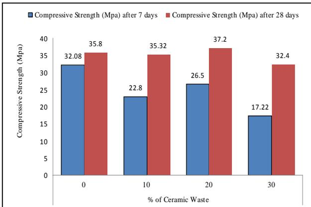
Figure 5. Test Result of Compressive Strength
