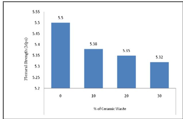
Figure 6. Flexural Strength (Mpa) after 28 days
