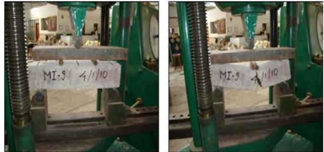
Figure 4. Flexural testing on samples
