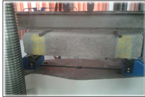
Figure 4. Flexural test setup of the RC beam
