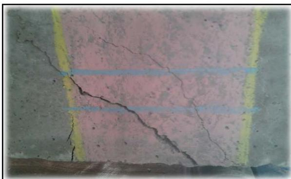
Figure 7. Crack pattern observed when lateral stirrups are provided in shear span
