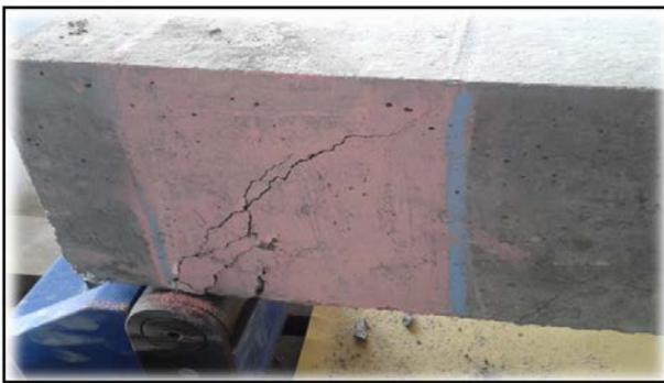
Figure 6. Crack pattern observed when vertical stirrups are provided in shear span
