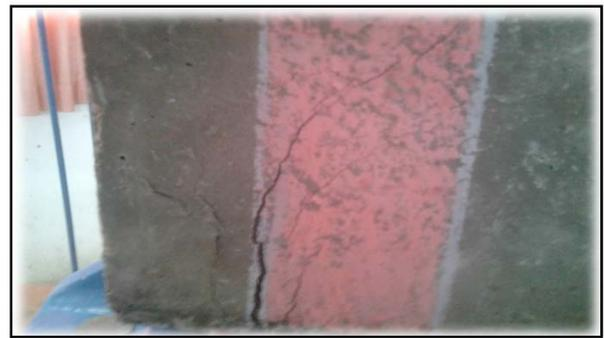
Figure 8. Crack pattern observed when inclined stirrups are provided in shear span
