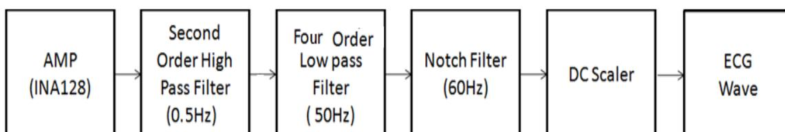
Figure 1. Flow diagram of ECG module for detecting ECG
