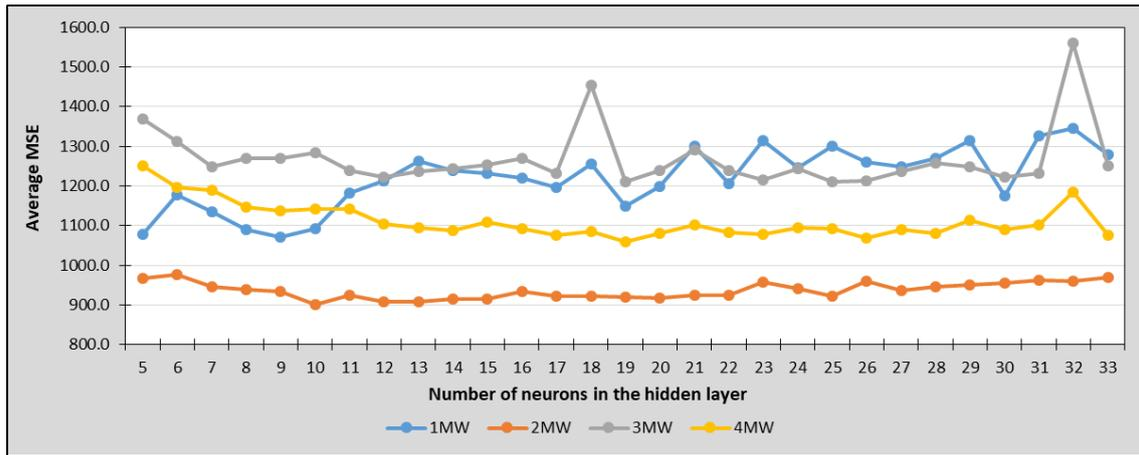
Figure 3. Average MSE of the validation set based on the moving window size for training
