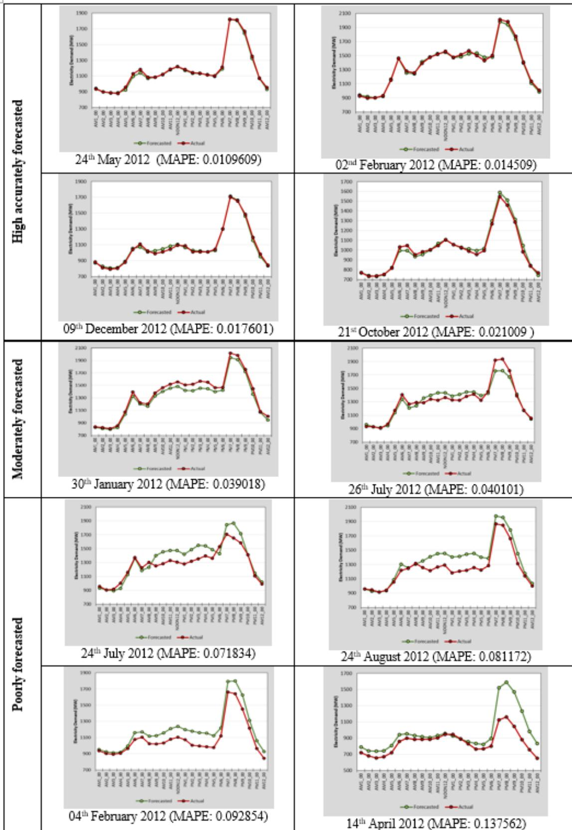
Figure 7. Some well, moderately and poorly forecasted days using the final iterative neural network
