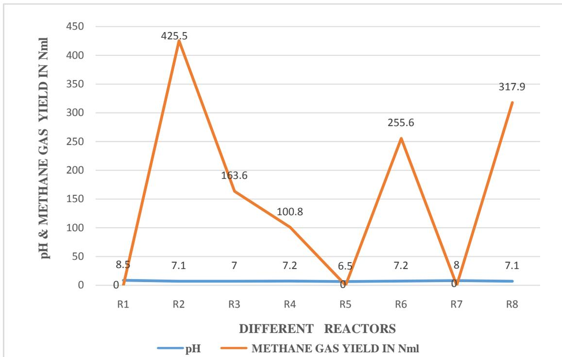
Figure 4. Effect of pH on Methane gas Yield in Different Reactors
