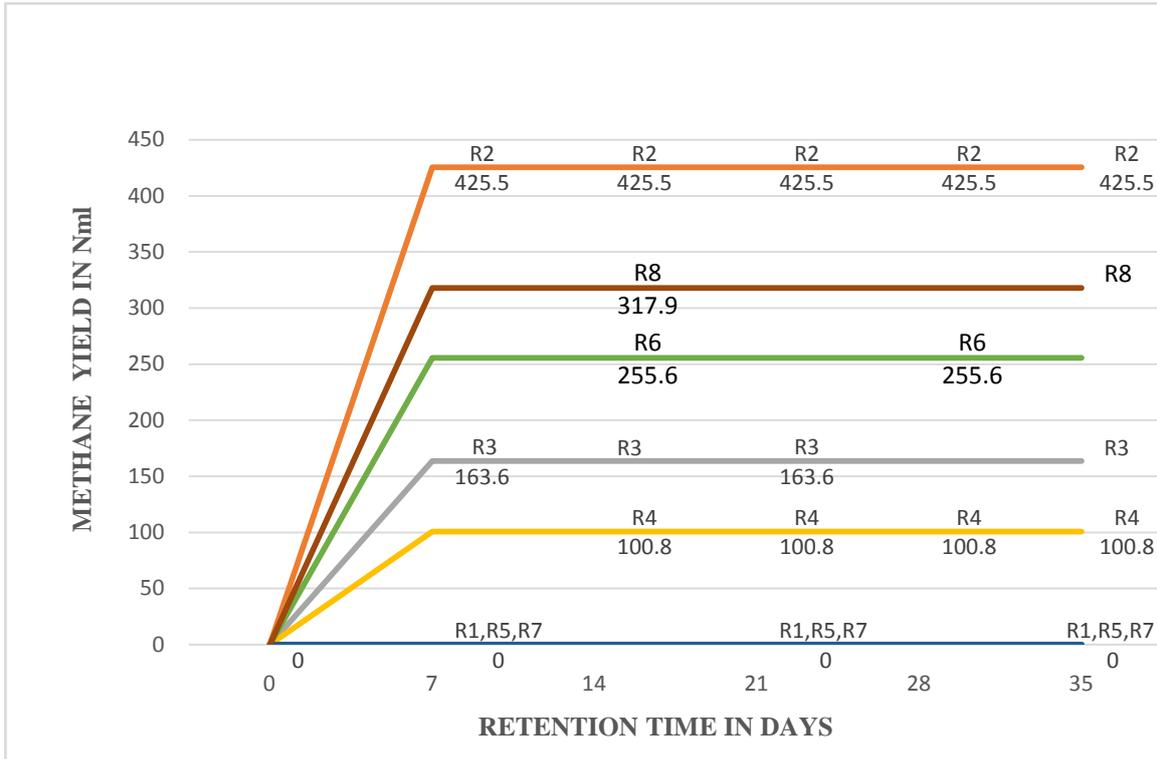
Figure 3. Effect of Retention Time on Methane gas Yield
