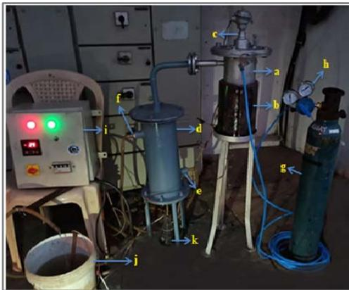
[a-Batch reactor; b-Heater; c-Sensor; d-Condenser; e-Water In; f-Water Out; g-Nitrogen (Purging Gas); h-Control Valve; i-PID controller; j-Water Tank; k-Liquid Collection Point].
