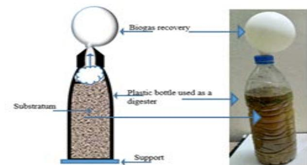
Figure 1. Diagram and photo of the digester
