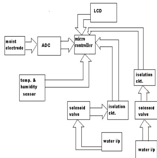
Figure 1. Block diagram for microcontroller based Drip irrigation system
